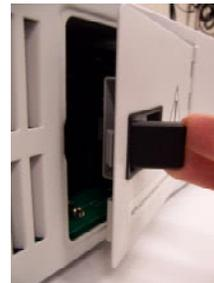
2. Close the bulb side door and verify that the bulb turns on but the light source stays in standby with the same displays on the LED.
