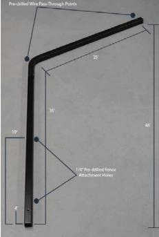
Once the brackets are firmly attached, the next step is to thread Guide Wire through the tip and junction of the brackets. These wires act as a support between brackets to help maintain a safe and uniform shape.
