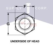
‡Length of a cap screw is measured from the underhead bearing surface to the extreme end of the screw.
