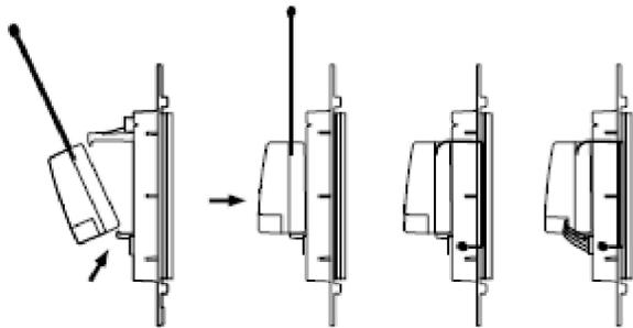
6. Connect the Nano device to WallSwipe using the provided JST 1.5mm connection cable. Make sure that the cable is fitted well into Nanos Touch Panel port and inserted the WallSwipe connection port.
