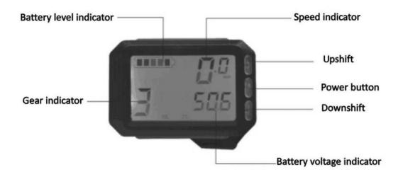
Press and hold the Power button to turn the speedometer ON/OFF.
