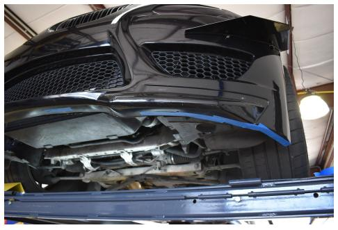
3. Hold your driver's side spat against the underside of the bumper. Align it so the back of the spat is flush with the edge of the fender well, and so the holes line up with the underside of the bumper. Hold steady and mark the rearmost hole. Drill that hole with your drill and ½" drill bit. (2 PICS)
