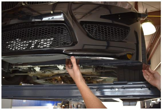
4. Loosely install your spat into the one hole with a 20mm long bolt pointing upward + fender washer, and ½" small washer + nyloc nut on top. Rotate the spat so the holes line up with the underside of the bumper and mark them with your pen or pencil. Remove the spat and drill all holes. Remove the tape and install your spat. The 30mm bolt + 15mm spacer will be placed at the front as shown in the following picture. Securely tighten. (ignore the extra holes we have) (2PICS)
