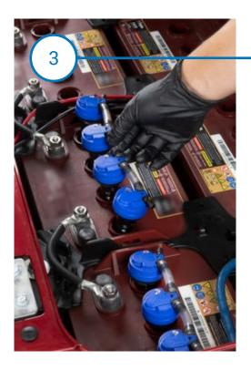
Insert the strings of valves into the cells. \*Do **not** snap into place.
