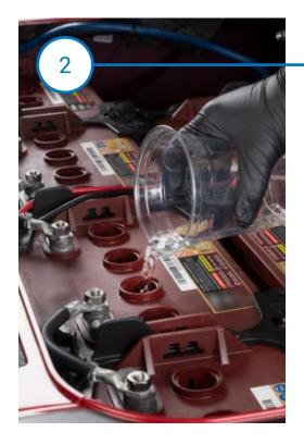
Ensure the electrolyte level is covering the plates in each cell. If not, add just enough water to cover the plates.
