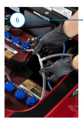
When all valve strings are connected, install the fill tube by cutting the tubing between two batteries. The fill tube should generally be placed in the center of the battery. Use the System Diagram for proper placement.
