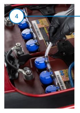
Attach the tubing onto the first string of valves. Make sure it is secure and covers the barbs completely.
