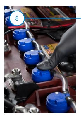
Lastly, push down on the center of each valve to snap into the cell.
