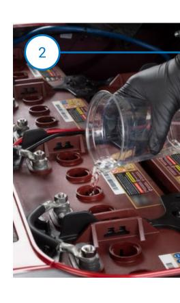
Ensure the electrolyte level is covering the plates in each cell. If not, add just enough water to cover the plates.
