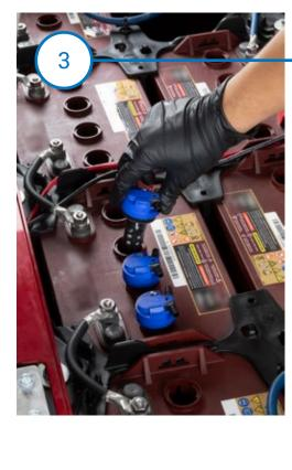
Make sure the valves are facing the same way on each individual battery.
