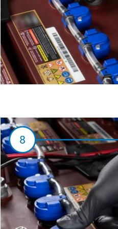
Lastly, push down on the center of each valve to snap into the cell.
