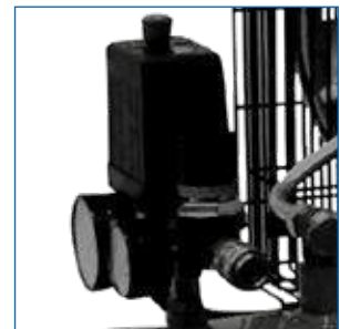
Output air regulators and quick coupling
