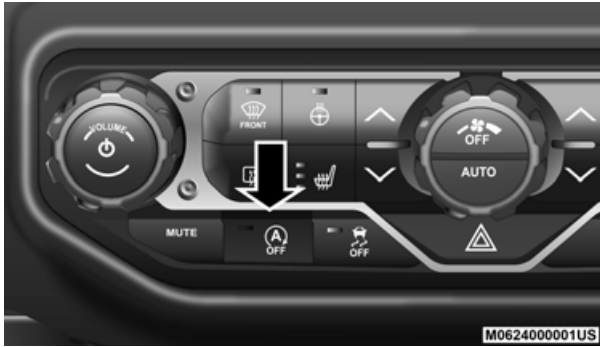
STOP/START Off Switch
