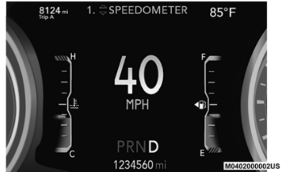
7.0 Inch Instrument Cluster Display Location
