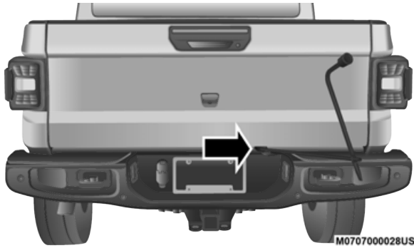
Inserting The Extension Tubes Into The Access Hole
