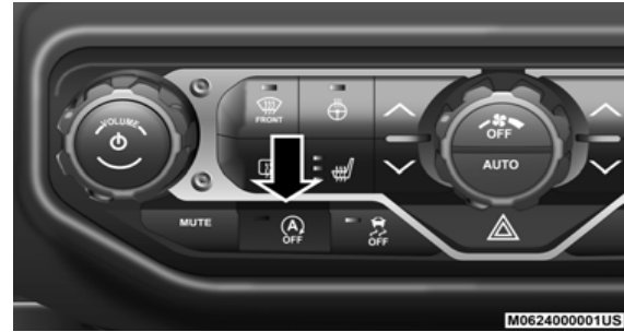
STOP/START Off Switch
