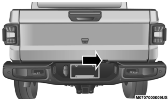
Access Hole Location
