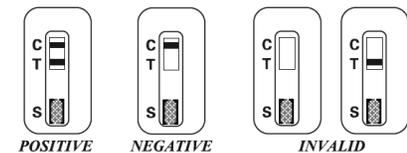
**NOTE:** Avoid over flooding the device with sample. This will cause erroneous result. If this occurred, it is strongly recommended that the test be repeated. Also, if the flow of the sample is not observed through the viewing window, this is due to an insufficient amount of urine sample dispensed into the sample well.
