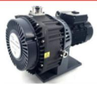
GWSP series oil free scroll vacuum pumps are based on two spiral cylinders, one offset and orbiting against the other with an offset of 180°, thus several crescent-shaped pockets of differing sizes are created. By means of an eccentric drive, the orbiting scroll is made to orbit about the fixed scroll, reducing the volume of the pockets and compressing gases from the outside towards the inside thereby pumping the gases from vacuum chamber.
