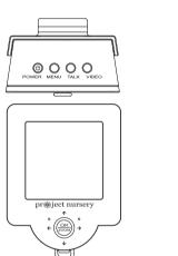
To turn the display on or off: Press the **VIDEO** button on the mini monitor.
