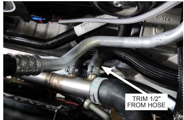
Fig. 3-g: Trim 1/2" From Suppl. Radiator Hose (Closest to driver side wheel well.)
