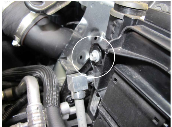
Fig. 1-ab: Remove Fan Shroud Screws (1 of 2 screws shown.)
