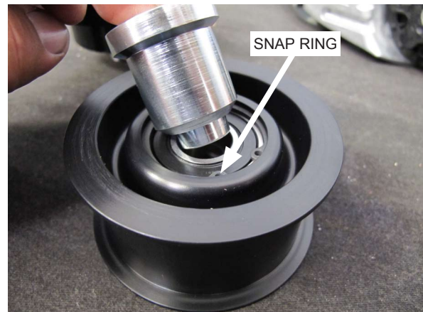
Fig. 4-j: Smooth Steel Idler Orientation
