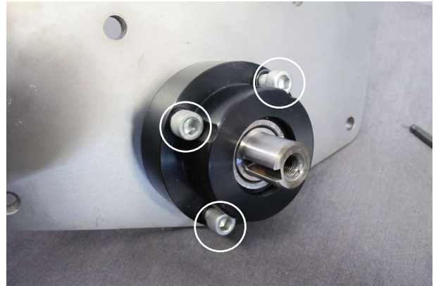
Fig. 1-p: Remove Jackshaft Assembly (3 of 4 screws shown.)
