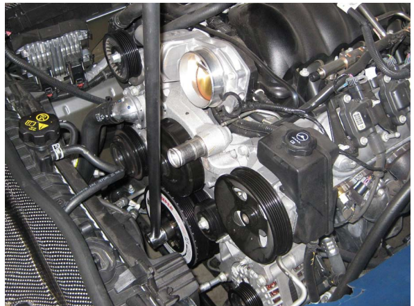
Fig. 2-b: Remove Damper Bolt (5th Gen Camaro shown.)
