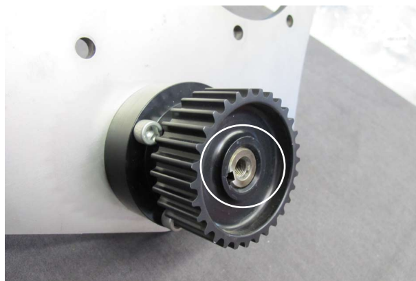
Fig. 1-o: Remove Pulley Retainers & Pulleys (Cog pulley shown. Repeat for 6-rib pulley.)
