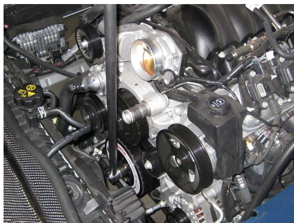
Fig. 2-g: Install & Torque Damper Bolt (5th Gen Camaro shown.)
