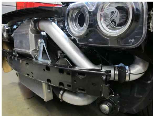
Fig. 6-ae: Install discharge tube 'B'
