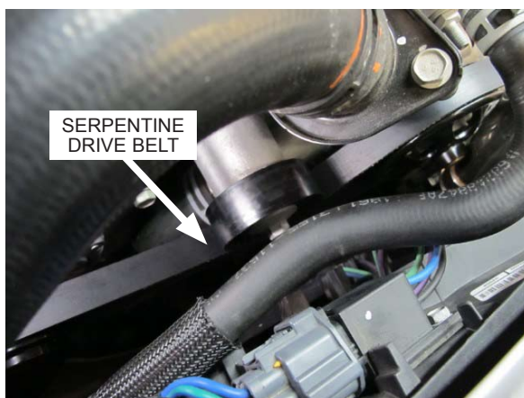
Fig. 5-i: Slide serpentine belt under OEM passenger side smooth idler pulley
