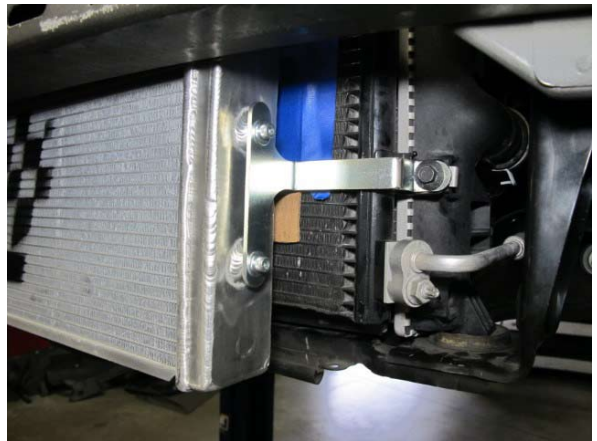
Fig. 6-k: Install driver side of heat exchanger assembly
