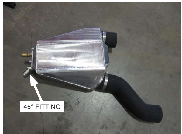
Fig. 6-x: Install silicone sleeves to air/water cooler as shown
