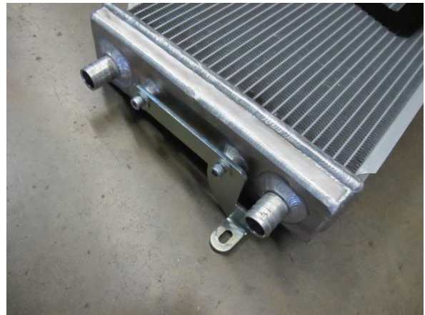
Fig. 6-h: Install passenger side heat exchanger bracket
