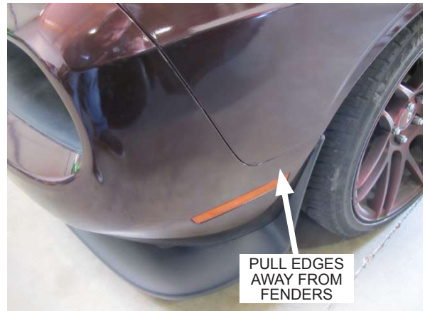
Fig. 2-j: Remove front bumper cover
