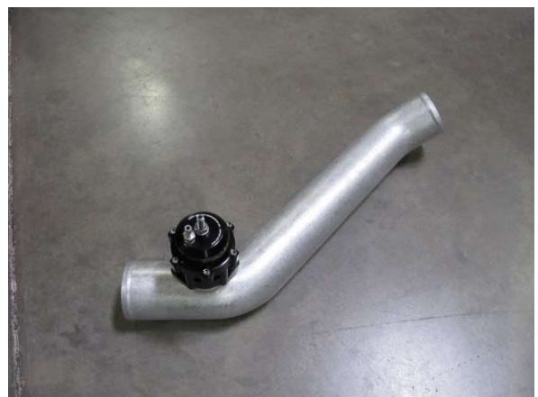
Fig. 6-ad: Install bypass valve to discharge tube 'B'
