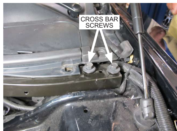
Fig. 1-c: Remove cross bar screws
