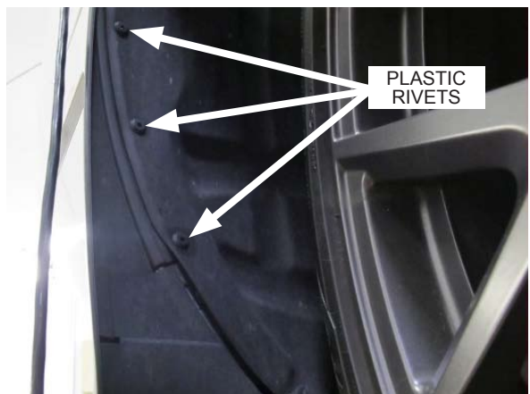
Fig. 10-c: Resecure using provided plastic rivets
