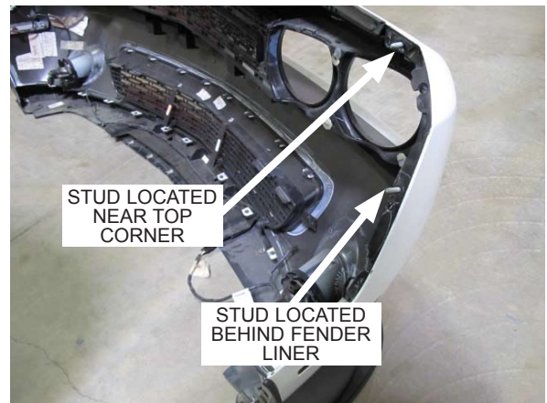
Fig. 2-h: Remove two nuts (Bumper removed for clarity)
