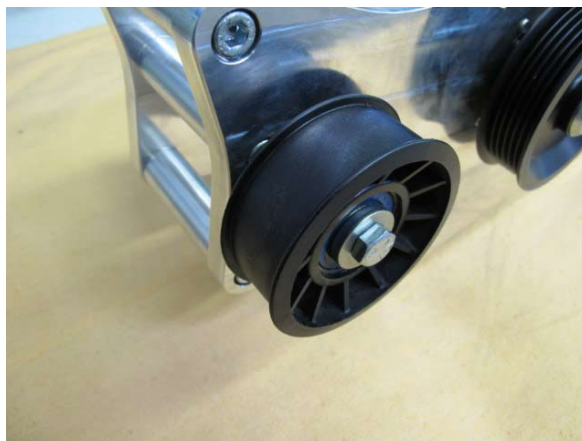
Fig. 5-b: Remove serpentine belt idler pulley
