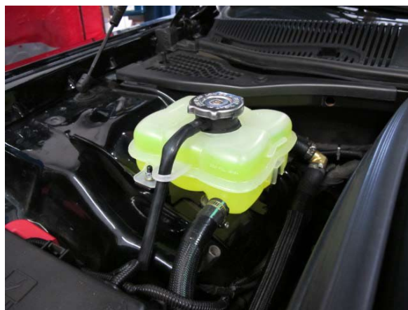
Fig. 8-z: Fill air/water cooling system with 50/50 water/coolant mix
