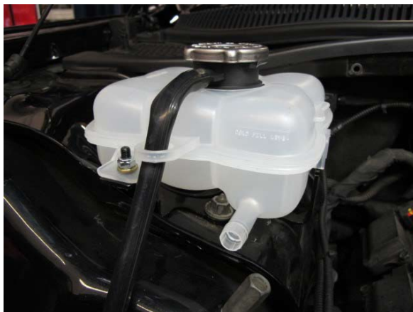
Fig. 8-m: Install air/water cooler system reservoir to mount
