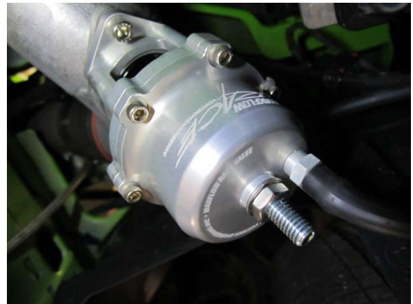
Fig. 7-k: Attach vacuum hose to bypass valve
