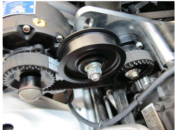
Fig. 7-d: Tension cog belt
