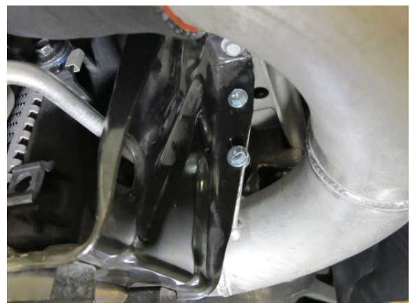
Fig. 6-aa: Secure discharge tube 'D' to lower radiator support
