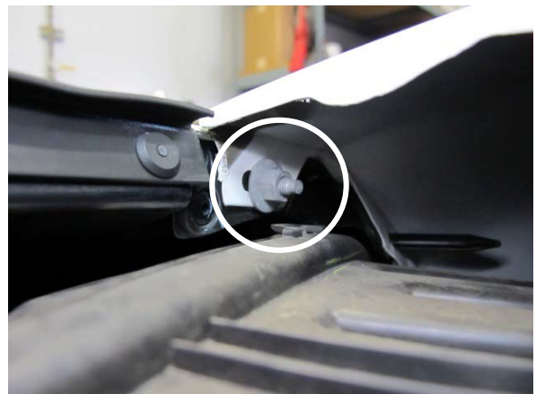
Fig. 2-f: Remove two nuts
