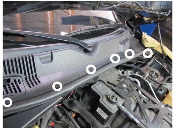
Fig. 1-b: Remove plastic fasteners
