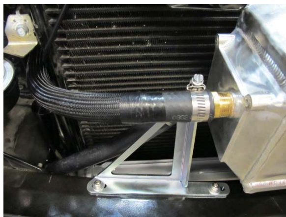
Fig. 8-u: Attach 3/4" coolant hose to air/water cooler
