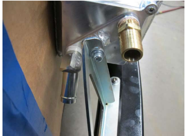
Fig. 6-s: Temporarily secure passenger side of air/water cooler
