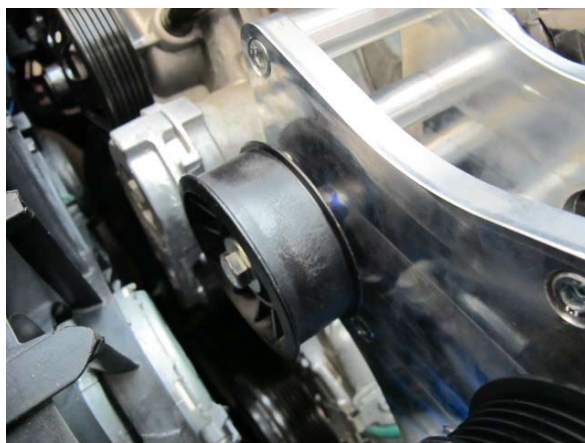
Fig. 5-h: Reinstall serpentine belt idler pulley
