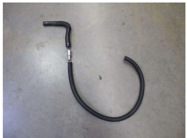
Fig. 7-f: Breather hose assembly
