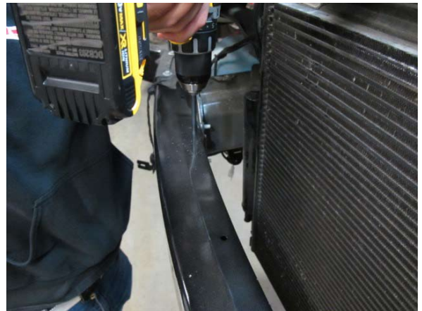
Fig. 6-q: Drill through two holes on front bumper support
