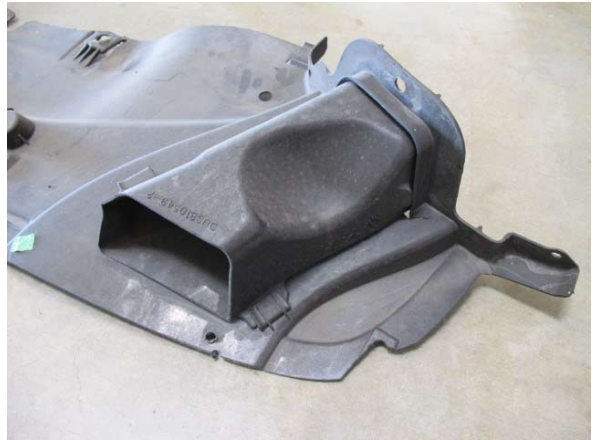
Fig. 10-a: Front brake cooling ducts
