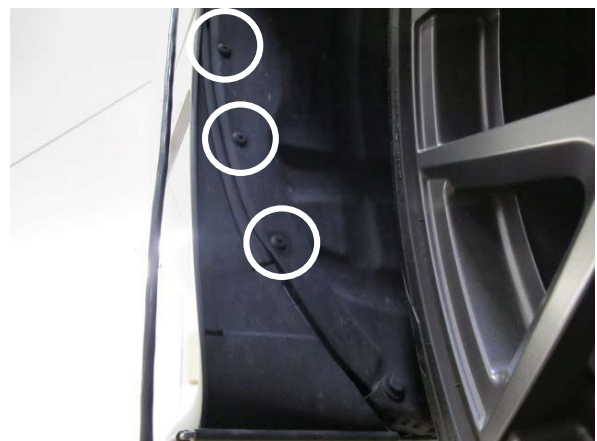
Fig. 2-c: Drill through and remove plastic rivets
