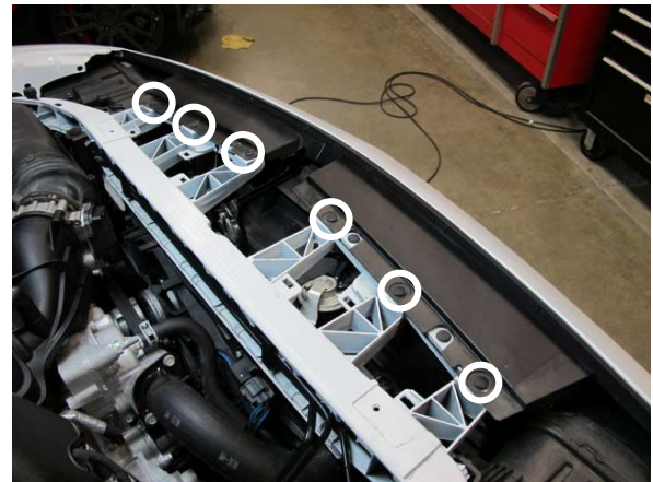
Fig. 2-b: Remove six plastic fasteners
