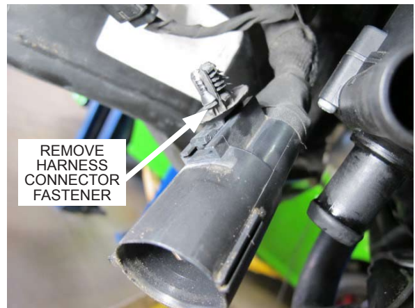
Fig. 8-e: Remove plastic harness connector fastener
