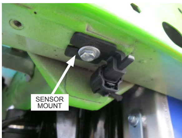
Fig. 6-ag: Reinstall ambient air temperature sensor as shown
