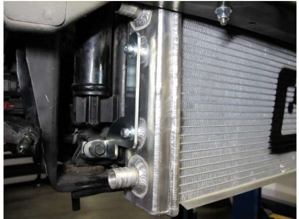
Fig. 6-j: Install passenger side of heat exchanger assembly
