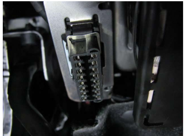
Fig. 11-e: Calibrator cable OBD II port installed
