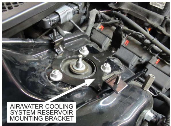
Fig. 8-l: Install air/water cooler system reservoir mount
