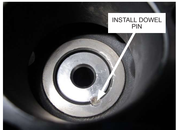
Fig. 3-e: Install dowel pin
