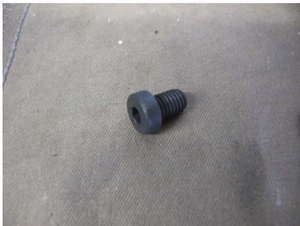
Fig. 8-h: Shorter front bumper support screw
