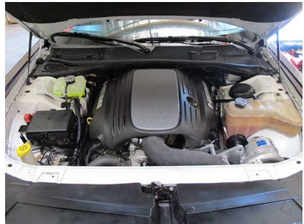
Fig. 10-e: Reinstall engine cover
