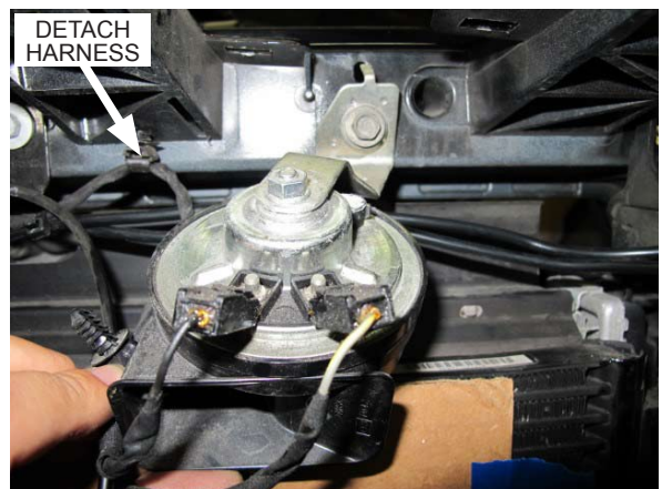
Fig. 6-l: Remove driver side horn
