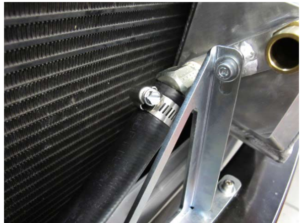
Fig. 8-k: Install long end of 150° molded hose to air/water cooler
