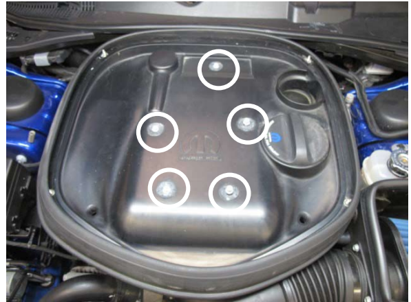
Fig. 2-p: Remove shaker base
