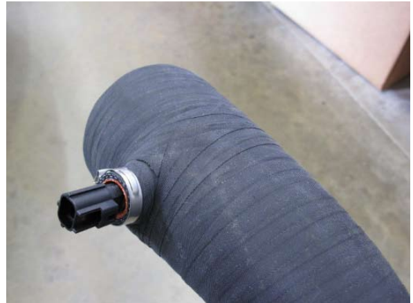
Fig. 6-ab: Install IAT sensor to molded boss on discharge sleeve 'E'
