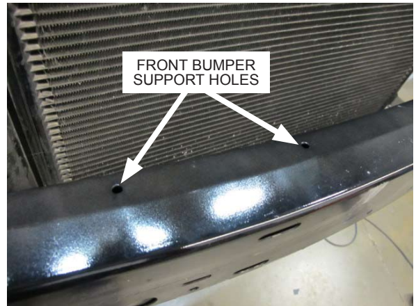
Fig. 6-p: 2x holes on front bumper support
