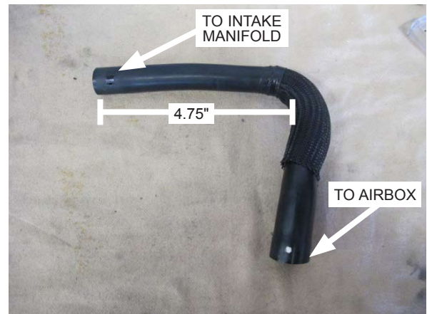
Fig. 7-e: Modify OEM breather hose
