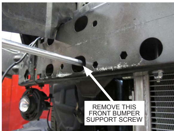
Fig. 8-g: Remove front bumper support screw
