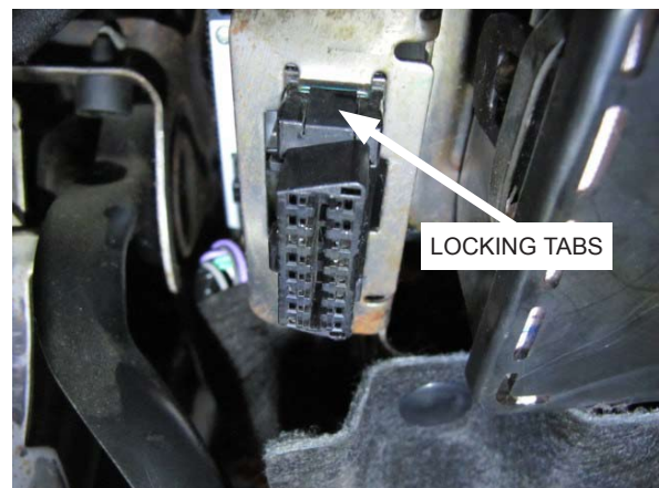
Fig. 11-c: Factory OBD II port locking tabs
