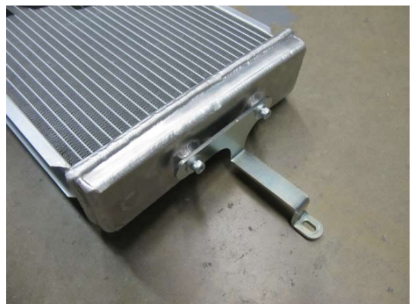
Fig. 6-i: Install driver side heat exchanger bracket
