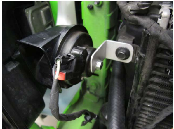
Fig. 6-n: Relocate driver side horn to upper radiator
