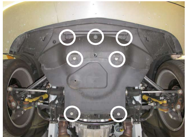
Fig. 2-e: Remove splash guard
