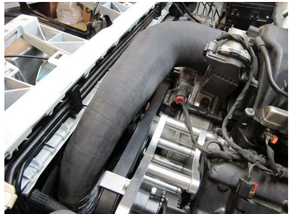
Fig. 6-ac: Install discharge sleeve 'E' and reconnect IAT sensor
