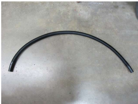
Fig. 8-n: 44" length of the 3/4" coolant hose
