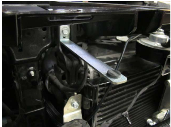
Fig. 9-b: 3/4" width radiator shroud bracket with rubber mount
