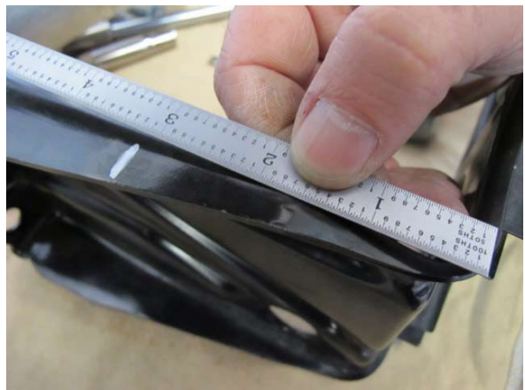
Fig. 4-c: Measure 3.25" from bottom edge
