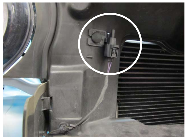
Fig. 2-l: Remove ambient air temperature sensor
