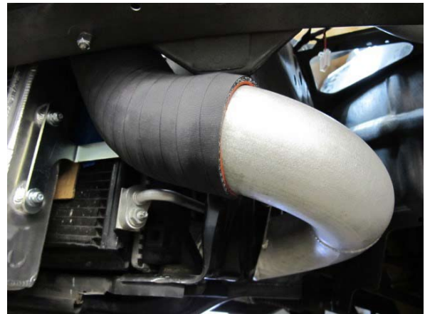
Fig. 6-z: Loosely install discharge tube 'D'
