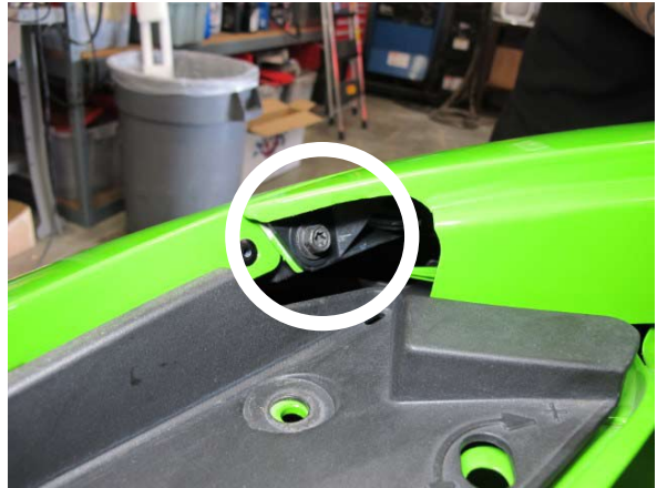
Fig. 2-g: Remove each upper front bumper cover screw
