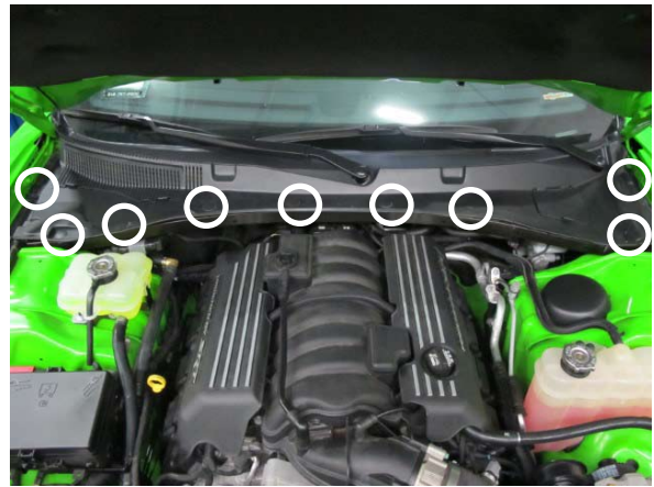
Fig. 1-b: Remove plastic fasteners
