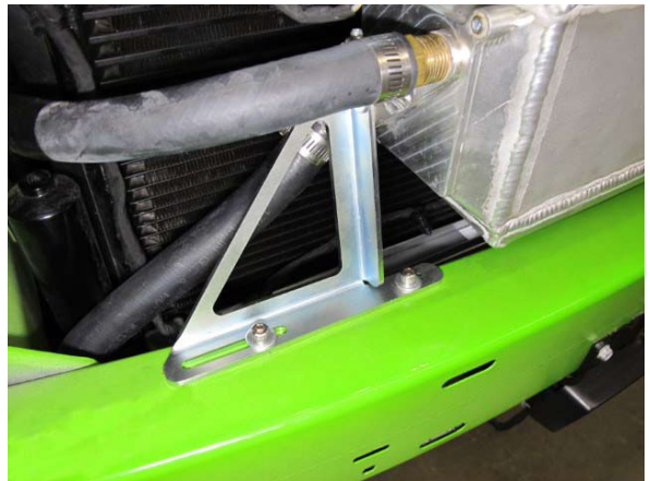
Fig. 6-z: Loosely install passenger side air/water cooler support bracket
