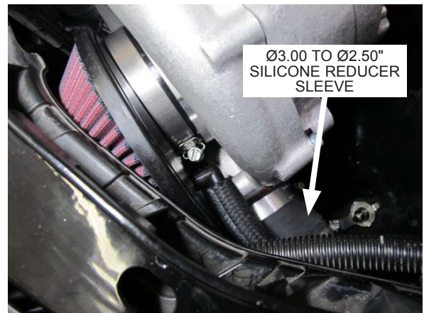
Fig. 7-h: Secure air filter and discharge tube A to supercharger
