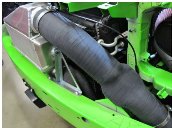
Fig. 6-ag: Install discharge sleeve 'B'
