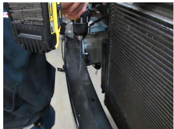
Fig. 6-u: Drill holes in front bumper support
