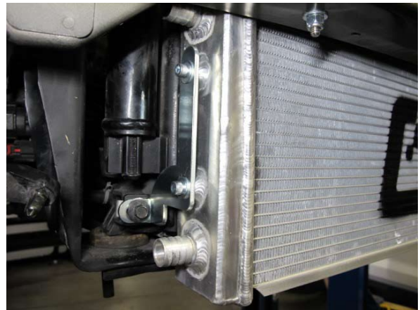
Fig. 6-k: Install passenger side of heat exchanger assembly
