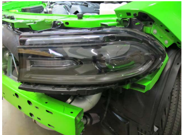
Fig. 6-af: Remove driver side headlight
