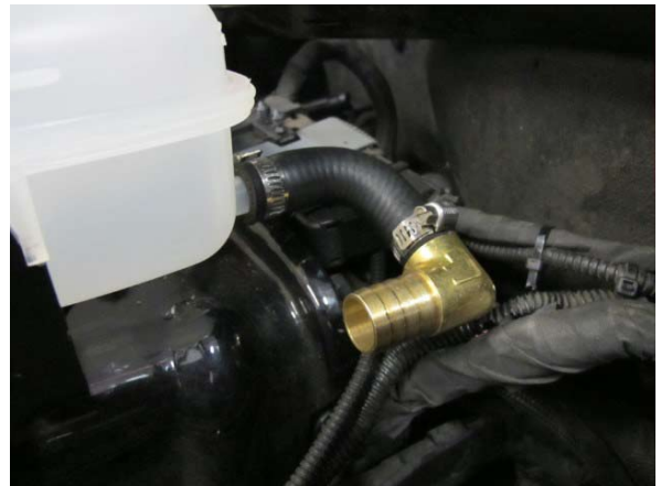
Fig. 8-q: Install hose and brass fitting assembly to air/water cooling system reservoir
