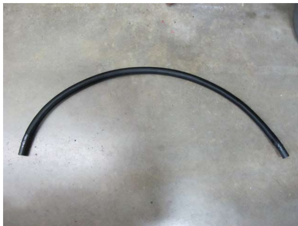
Fig. 8-n: 44" length of the 3/4" coolant hose
