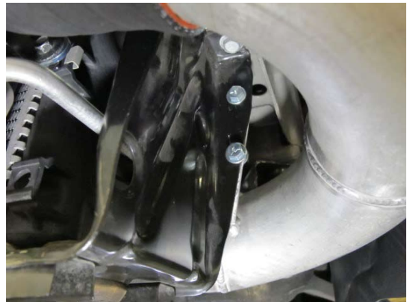
Fig. 6-ac: Secure discharge tube 'D' to lower radiator support
