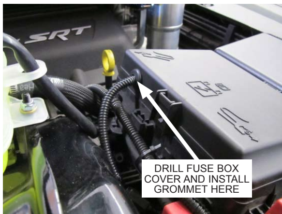
Fig. 8-b: Drill fuse box cover, install grommet and route wire into fuse box
