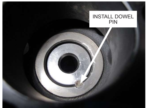
Fig. 3-e: Install dowel pin
