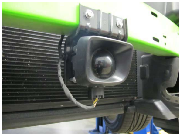
Fig. 2-i: Disconnect adaptive cruise control sensor
