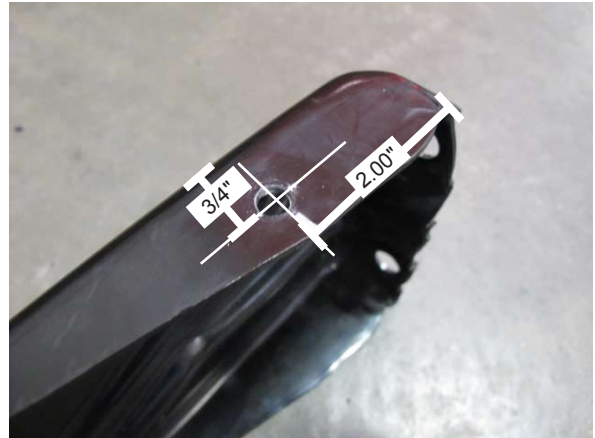
Fig. 4-g: Drill hole on passenger side rear edge of lower radiator support
