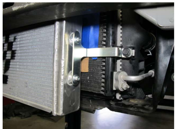
Fig. 6-l: Install driver side of heat exchanger assembly
