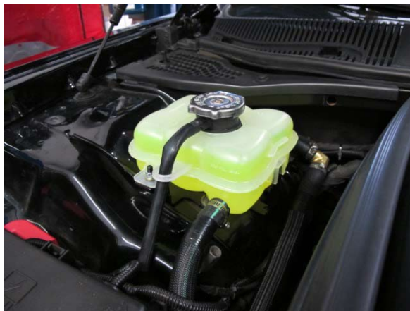
Fig. 8-z: Fill air/water cooling system with 50/50 water/coolant mix
