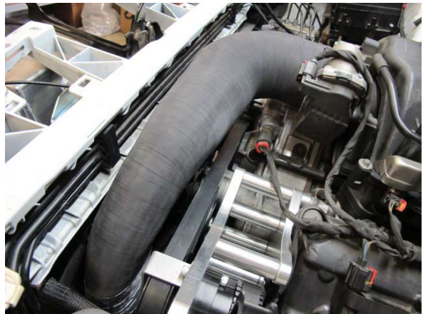
Fig. 6-ae: Install discharge sleeve 'E' and reconnect IAT sensor
