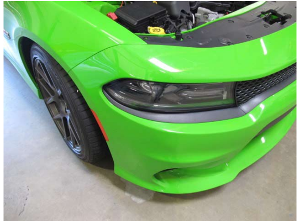
Fig. 9-a: Reinstall front bumper cover
