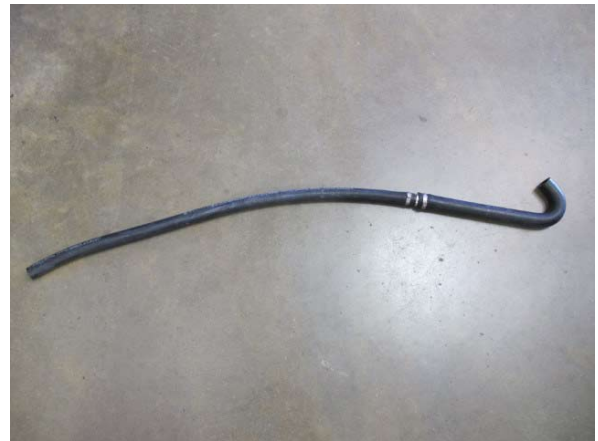
Fig. 8-w: 3/4" x 150° to 1/2" coolant hose assembly
