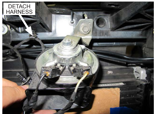
Fig. 6-m: Remove driver side horn
