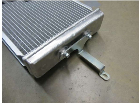
Fig. 6-j: Install driver side heat exchanger bracket
