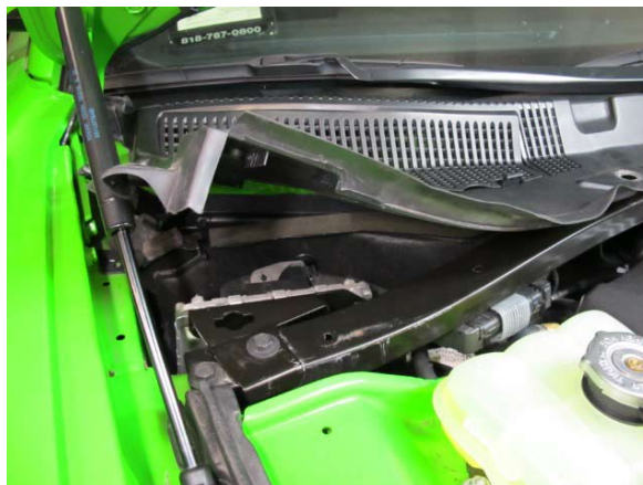
Fig. 1-d: Lift up passenger side of windshield cowl
