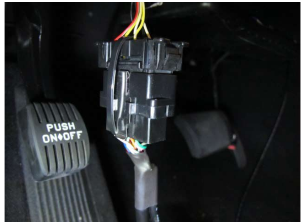
Fig. 10-d: Secure calibrator cable to factory OBD II port
