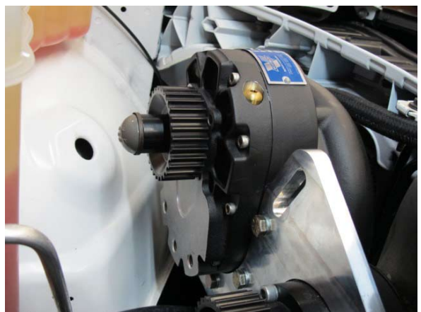
Fig. 7-c: Install supercharger to supercharger mounting bracket assembly
