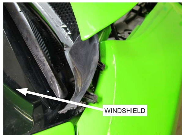
Fig. 1-c: Detach windshield cowl from passenger side fender
