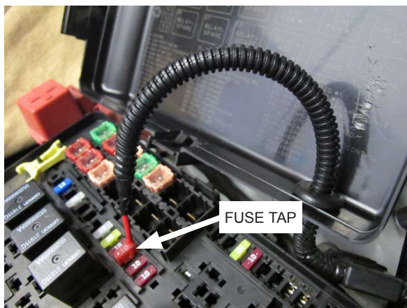
Fig. 8-c: Install fuse from water pump harness as shown
