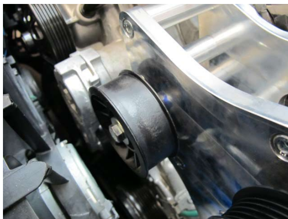
Fig. 5-h: Reinstall serpentine belt idler pulley
