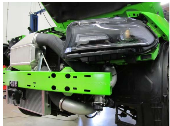
Fig. 7-i: Secure discharge tubes and discharge sleeves
