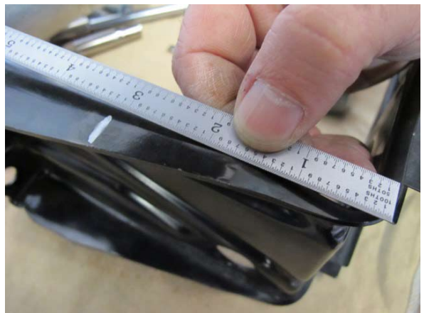
Fig. 4-c: Measure 3.25" from bottom edge
