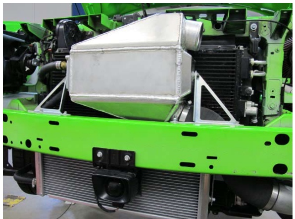
Fig. 6-aa: Install air/water cooler
