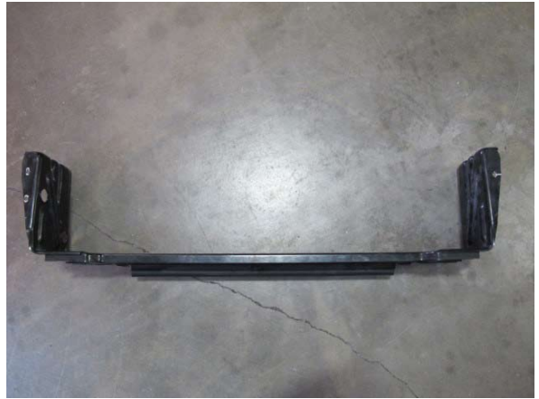
Fig. 4-b: Lower radiator support
