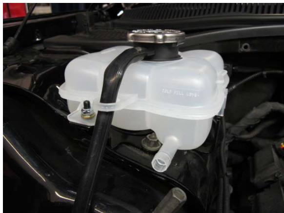
Fig. 8-m: Install air/water cooler system reservoir to mount
