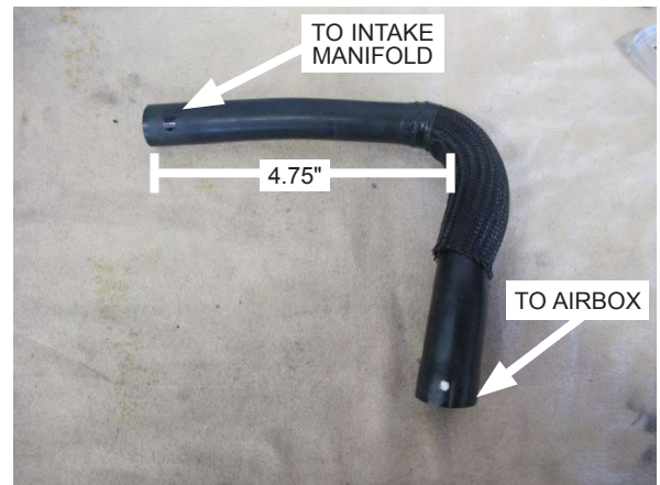
Fig. 7-e: Modify OEM breather hose
