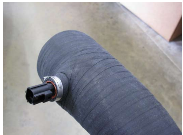
Fig. 6-ad: Install IAT sensor to molded boss on discharge sleeve 'E'
