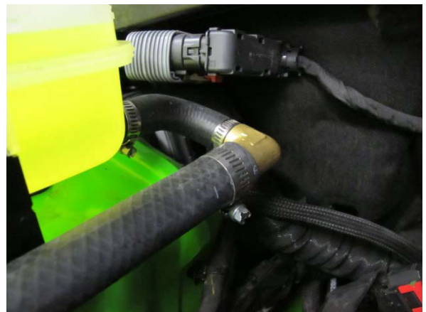
Fig. 8-r: Attach 44" length of 3/4" coolant hose to the brass fitting as shown
