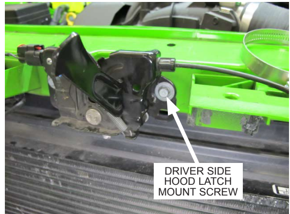
Fig. 6-p: Remove driver side hood latch mount screw
