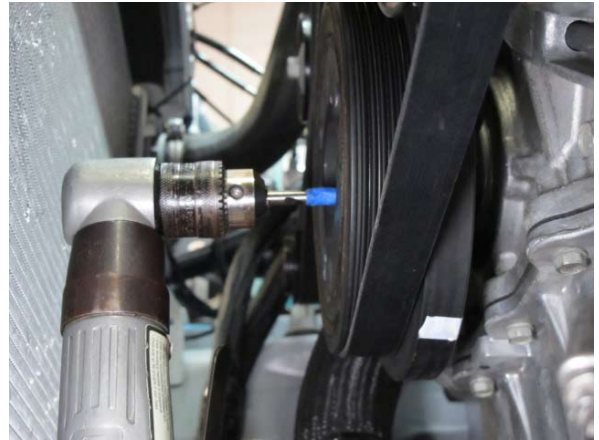
Fig. 3-d: Drill crankshaft / damper assembly
