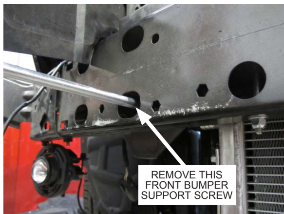
Fig. 8-g: Remove front bumper support screw
