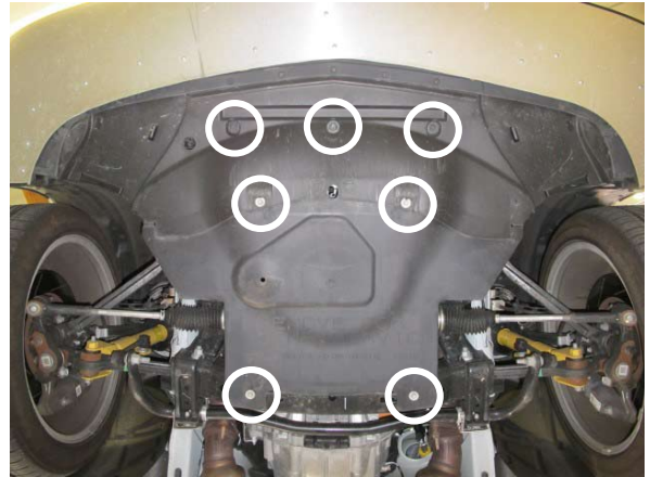
Fig. 2-d: Remove engine service panel fasteners
