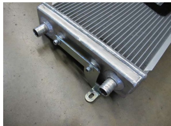
Fig. 6-i: Install passenger side heat exchanger bracket
