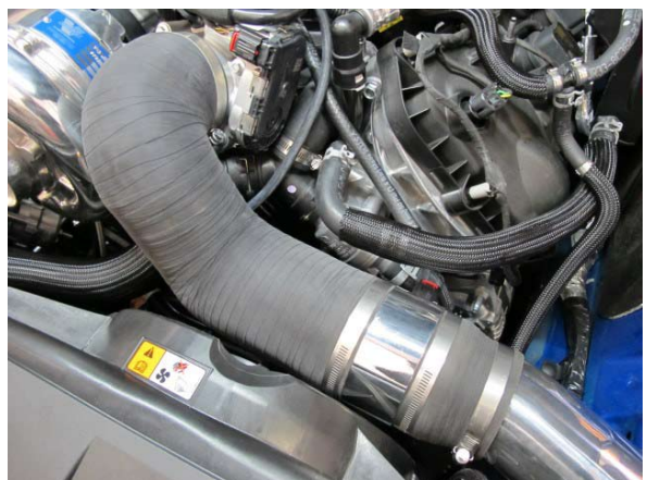
Fig. 6-ap: Secure all hose clamps
