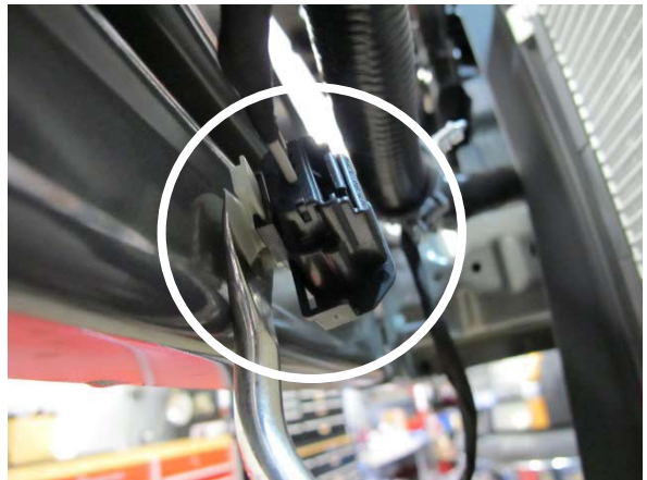
Fig. 6-n: Remove unused plug from front bumper support
