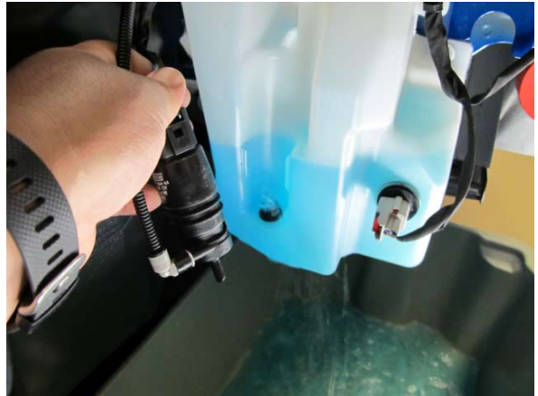
Fig. 6-d: Drain windshield washer fluid reservoir
