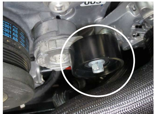
Fig. 2-q: Install offset smooth idler pulley and secure using OEM screw only
