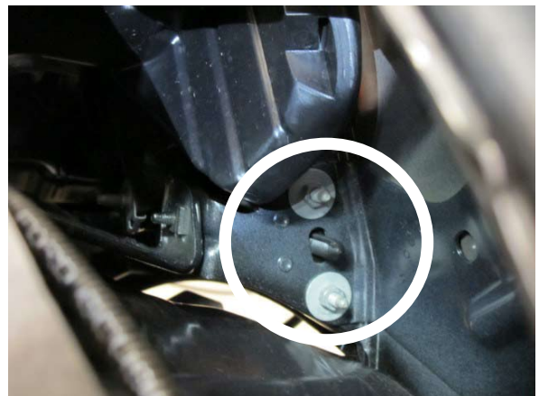
Fig. 1-i: Remove corner bracket fasteners
