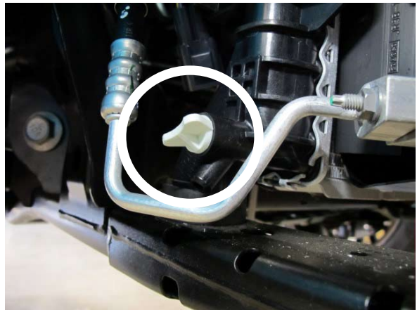
Fig. 1-w: Drain engine coolant
