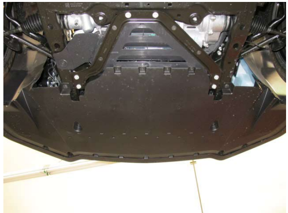
Fig. 1-k: Remove lower splash guards
