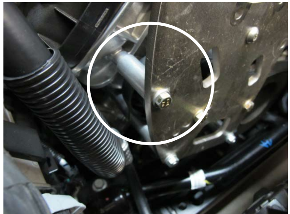
Fig. 2-k: Install 1x 1.928" and 1x .280" spacers
