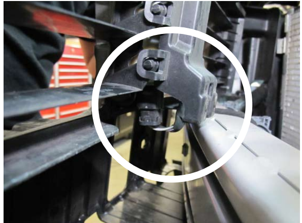
Fig. 1-s: Unplug motor & remove active grille shutter assembly
