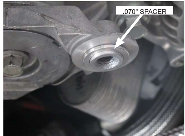
Fig. 2-p: Install .070" spacer onto pilot
