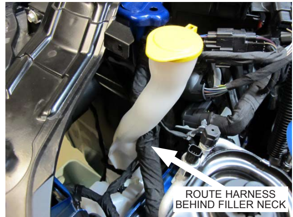
Fig. 6-k: Reinstall windshield washer fluid reservoir
