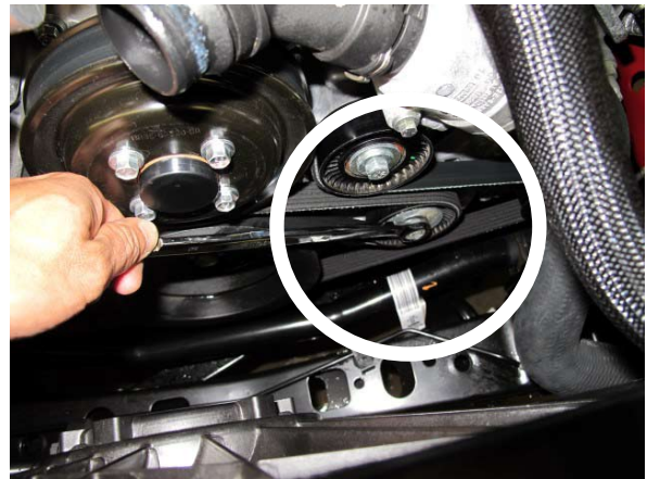
Fig. 1-z: Remove accessory drive belt
