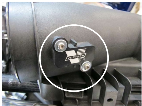
Fig. 7-f: Install MAF block-off plate
