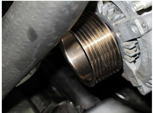
Fig. 2-t: Install provided 8-rib alternator pulley
