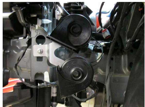
Fig. 6-ad: Remove horn assembly
