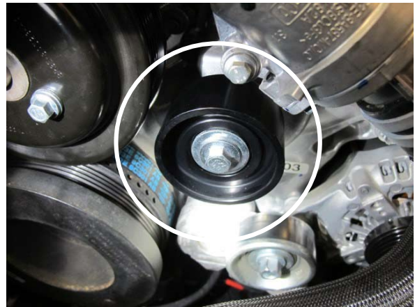
Fig. 2-n: Install smooth idler pulley and secure using OEM screw and washer
