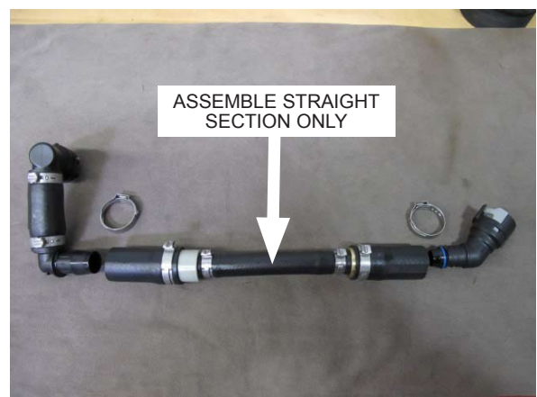
Fig. 7-c: Assemble straight section of PCV assembly
