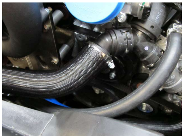
Fig. 4-l: Secure quick-release to hose using #24 hose clamp
