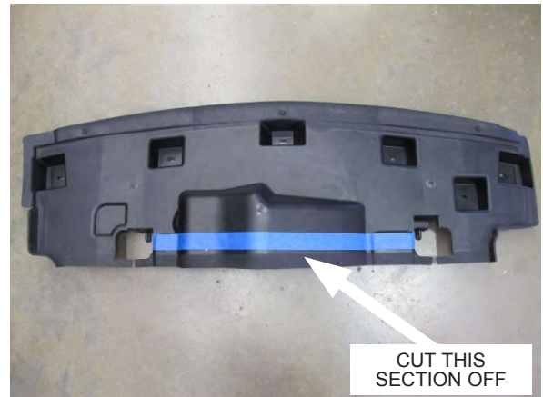
Fig. 6-ab: Modify upper radiator shroud
