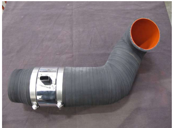
Fig. 6-ao: Assemble MAF sensor housing & sleeves as shown
