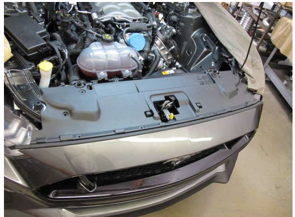
Fig. 1-d: Remove radiator support cover
