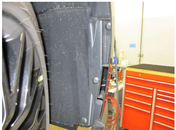
Fig. 1-f: Remove fender liner fasteners
