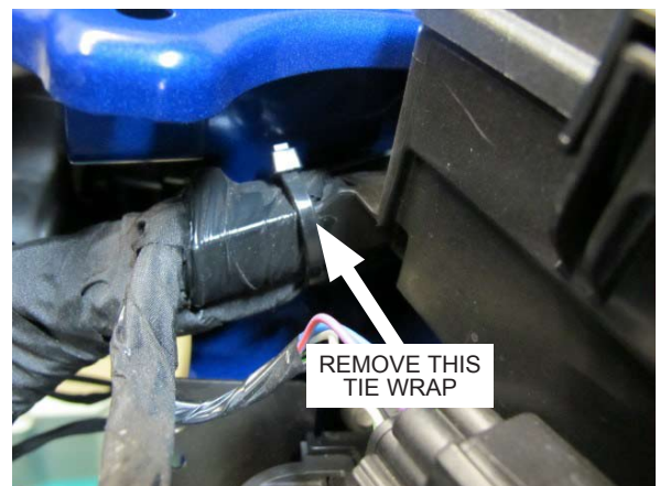
Fig. 6-i: Remove harness tie wrap
