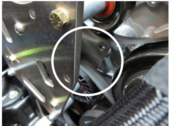
Fig. 3-a: Remove these spacers and hardware
