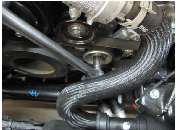
Fig. 3-g: Install supercharger drive belt
