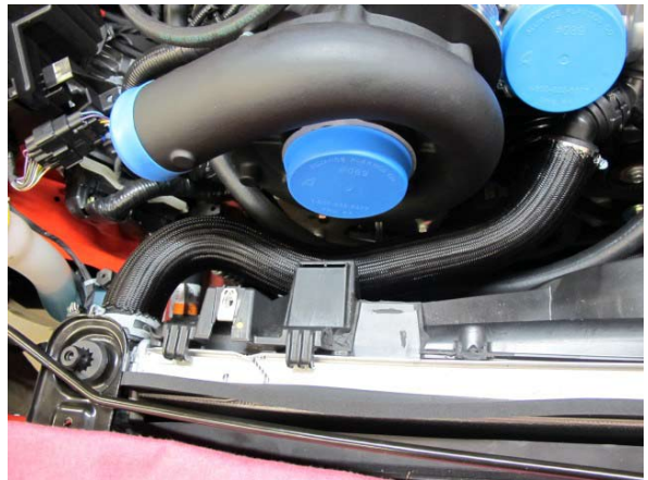
Fig. 4-k: Upper radiator hose (New configuration)
