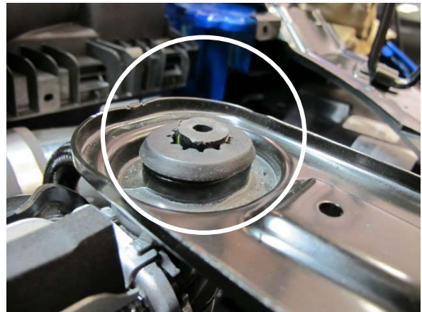
Fig. 7-n: Modify radiator mounting tabs
