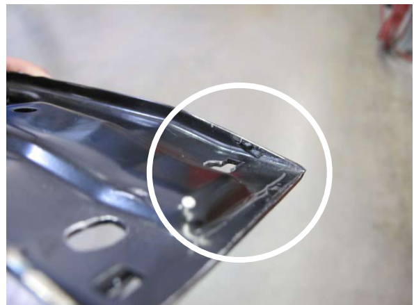
Fig. 4-f: Grind down raised edges to a taper
