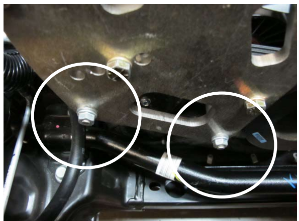
Fig. 2-l: Install 2x M8 nuts and 2x 5/16" washers
