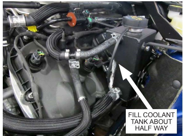
Fig. 4-y: Refill cooling system
