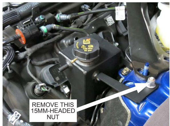
Fig. 4-r: Loosely attach coolant tank
