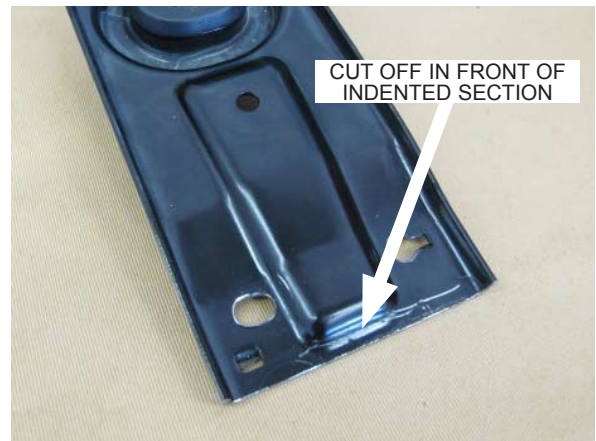
Fig. 4-e: Cut the upper radiator bracket as shown
