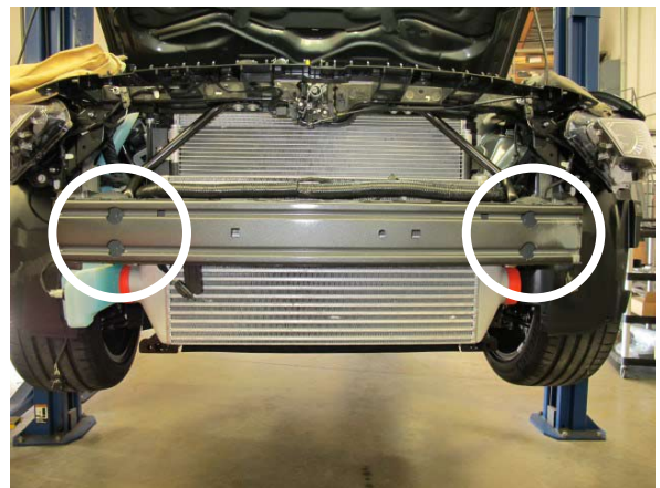
Fig. 6-x: Charge air cooler installation
