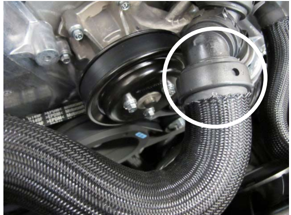
Fig. 4-j: Remove plastic hose clamp
