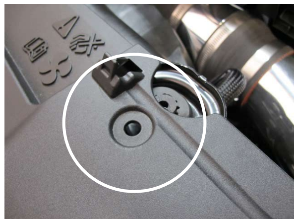
Fig. 7-o: Check upper radiator support cover
