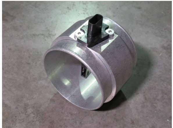
Fig. 6-an: Install MAF tensor to MAF housing
