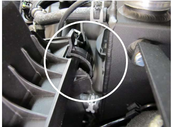
Fig. 7-g: Trim air box as necessary
