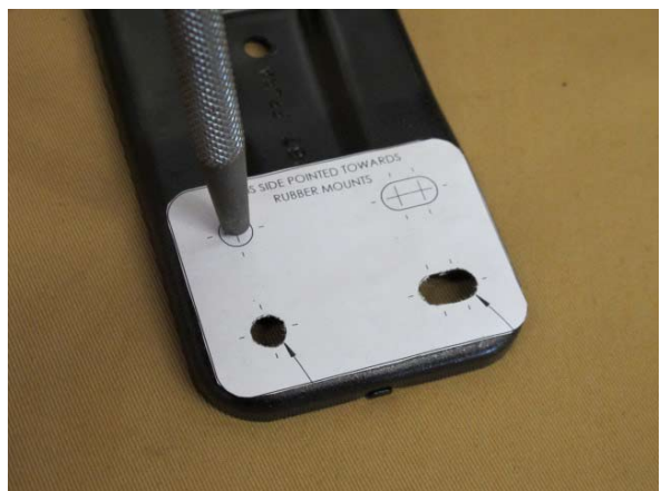
Fig. 4-c: Center punch the holes to be drilled
