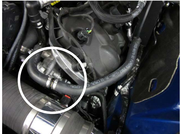
Fig. 4-v: OEM 3/4" coolant hose (Modified)
