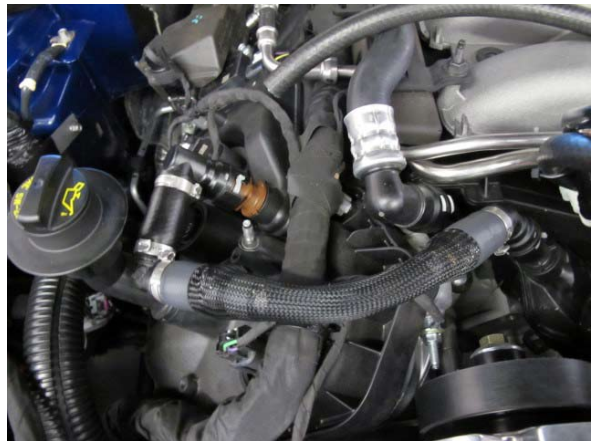
Fig. 7-e: Install PCV assembly
