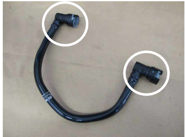
Fig. 7-a: Remove both quick-release fittings
