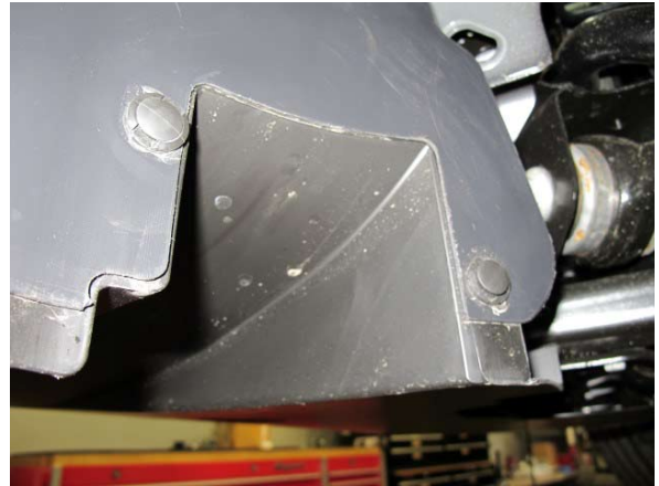
Fig. 1-g: Remove plastic fasteners
