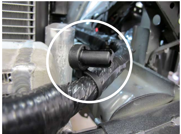
Fig. 6-q: Remove plastic harness clip
