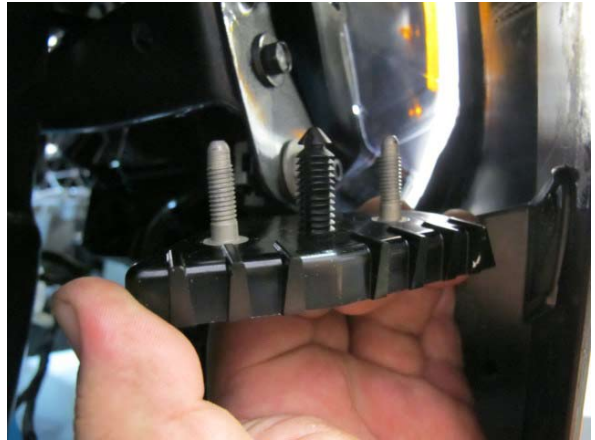
Fig. 1-j: Remove corner brackets
