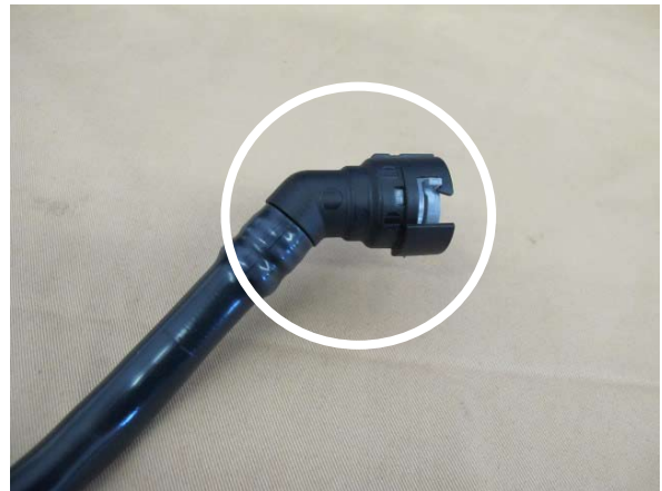
Fig. 7-b: Remove 45° quick-release fitting
