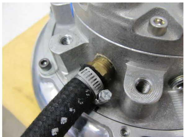
Fig. 3-c: Install oil drain hose
