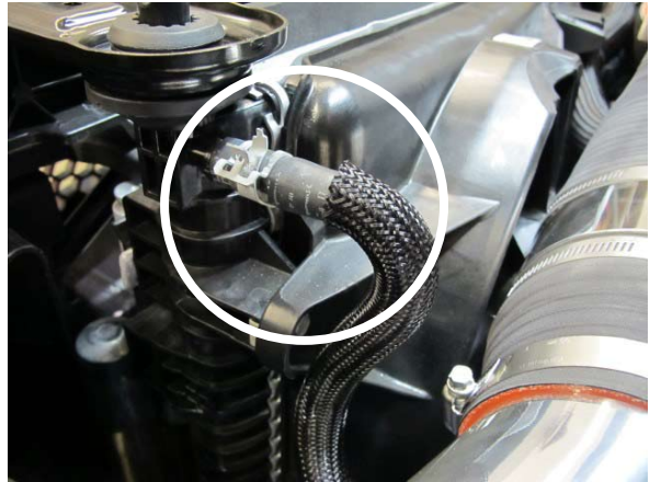
Fig. 4-m: Rotate the driver side OEM molded coolant hose 90°
