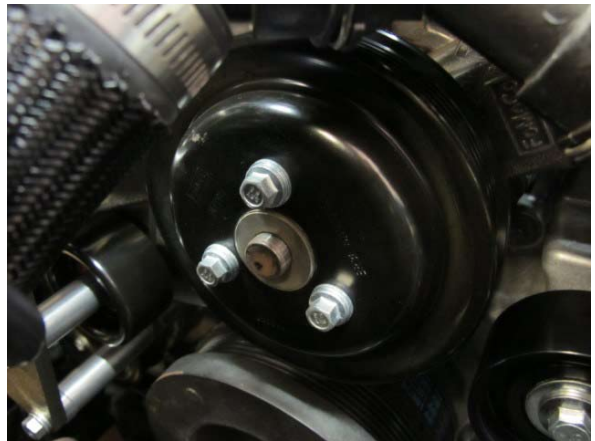
Fig. 3-h: Secure water pump pulley screws
