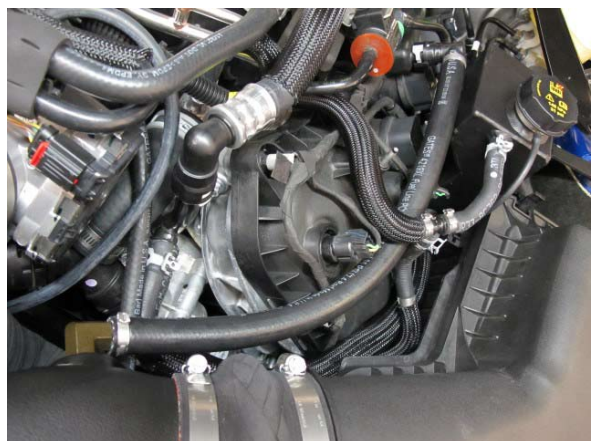
Fig. 7-i: Attach breather hose to air inlet
