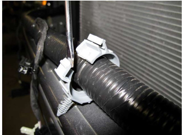
Fig. 6-p: Remove gray wire harness clips
