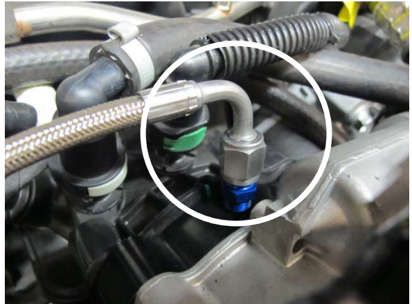
Fig. 6-aq: Attach vacuum hose to fitting
