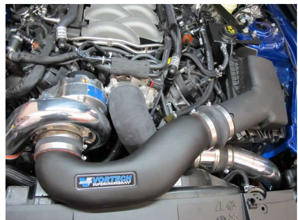
Fig. 7-l: Loosely install air inlet tube
