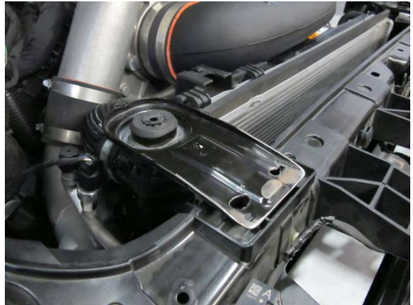
Fig. 4-g: Reinstall modified upper radiator brackets
