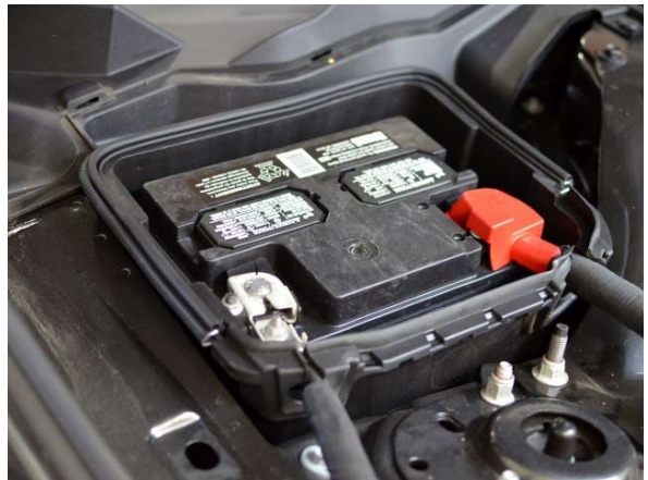
Fig. 1-b: Unplug battery leads
