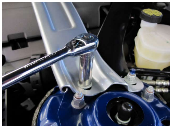
Fig. 1-c: Remove strut tower brace
