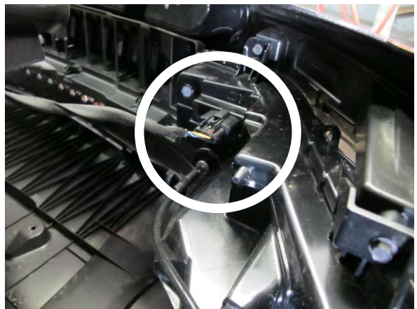
Fig. 1-l: Unplug bumper lights
