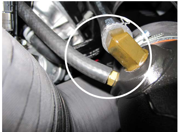
Fig. 7-m: Install 3/8" hose, then secure air inlet tube
