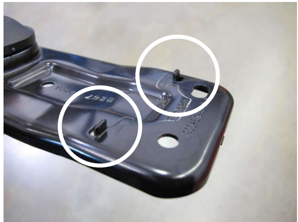
Fig. 4-b: Remove 2x protruding tabs
