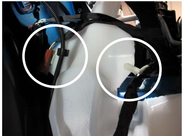
Fig. 6-e: Detach electrical harnesses & windshield washer fluid line
