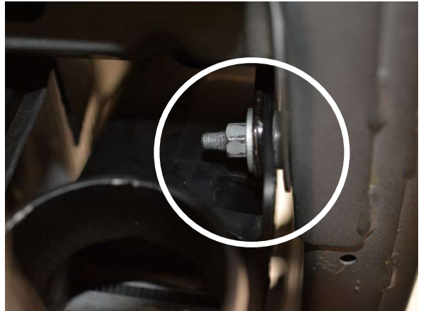
Fig. 6-y: Secure charge air cooler
