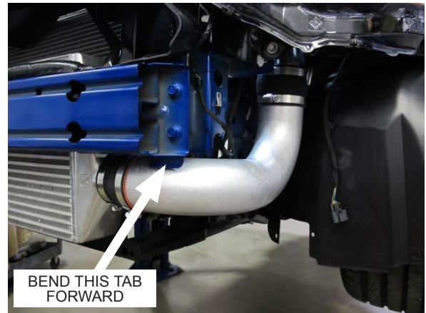
Fig. 6-al: Install discharge tube C
