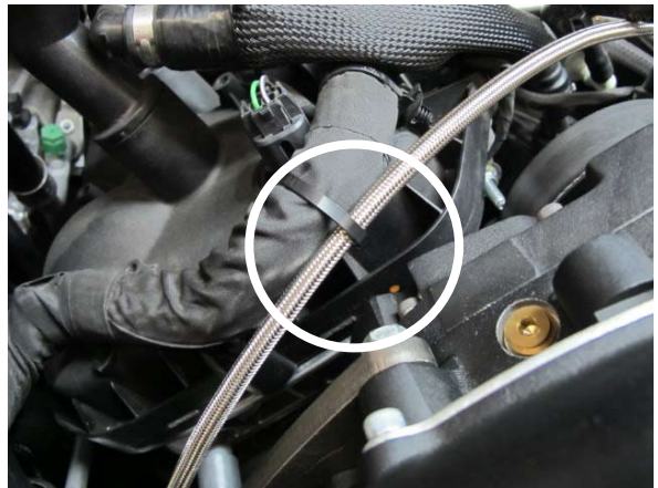
Fig. 6-ar: Secure stainless steel braided hose
