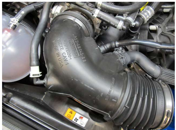
Fig. 1-u: Remove OEM air inlet
