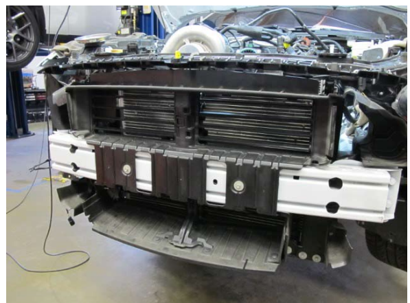
Fig. 1-o: Remove 8mm-headed fasteners
