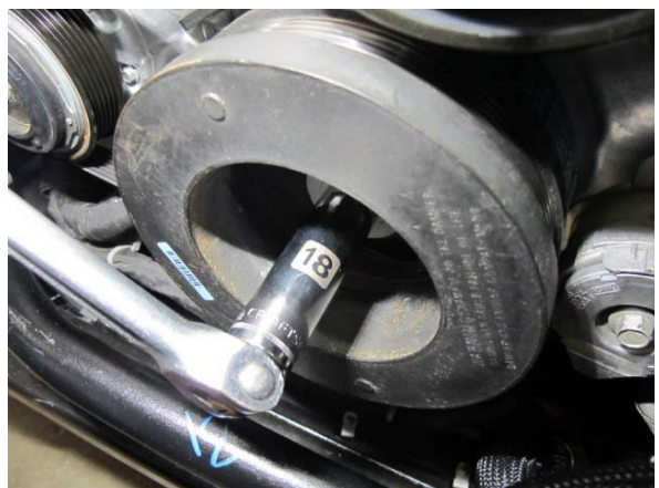
Fig. 2-u: Follow damper removal instructions included with your choice of damper
