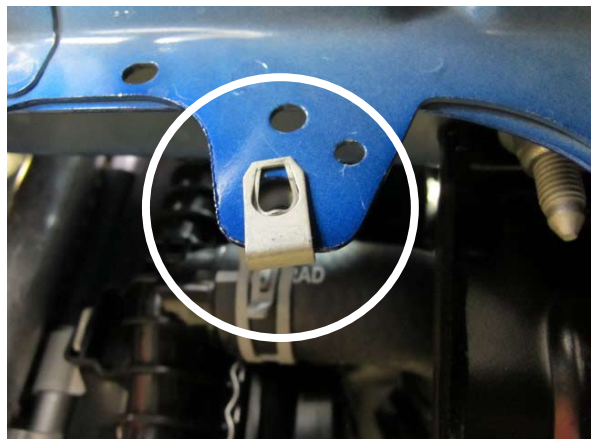
Fig. 6-as: Relocate OEM threaded clip
