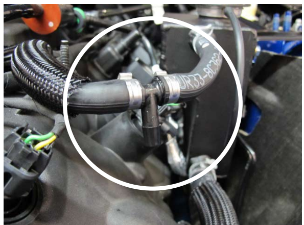
Fig. 4-x: Secure 3/8" plastic tee
