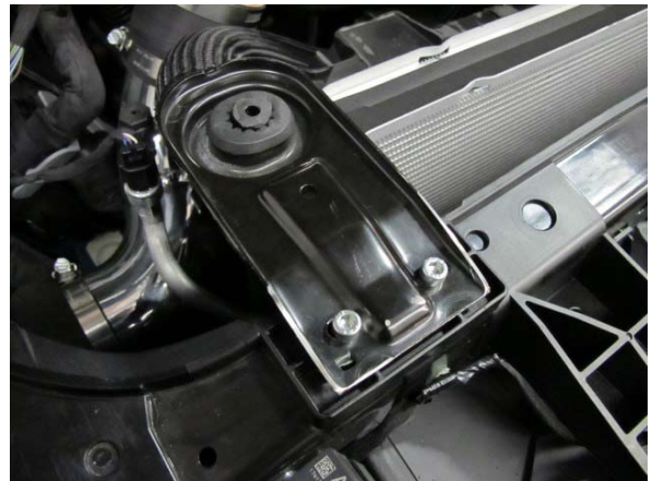
Fig. 6-au: Reinstall modified upper radiator brackets
