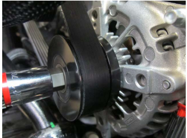
Fig. 2-s: Remove 6-rib alternator pulley
