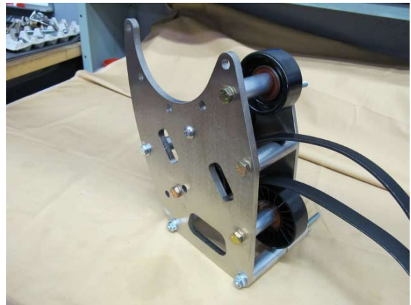
Fig. 2-b: Inspect supercharger mounting bracket assembly
