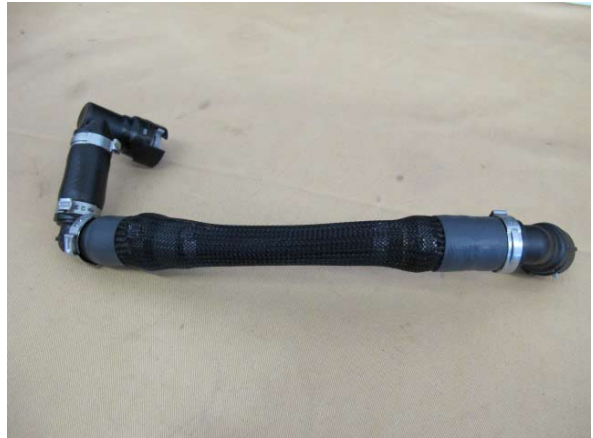
Fig. 7-d: Loosely assemble OEM quick-release fittings as shown
