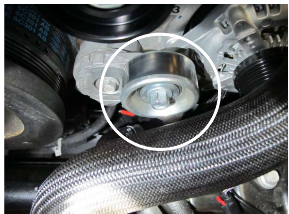
Fig. 2-o: Remove OEM smooth idler pulley located on belt tensioner
