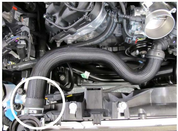
Fig. 4-i: Upper radiator hose (OEM configuration)
