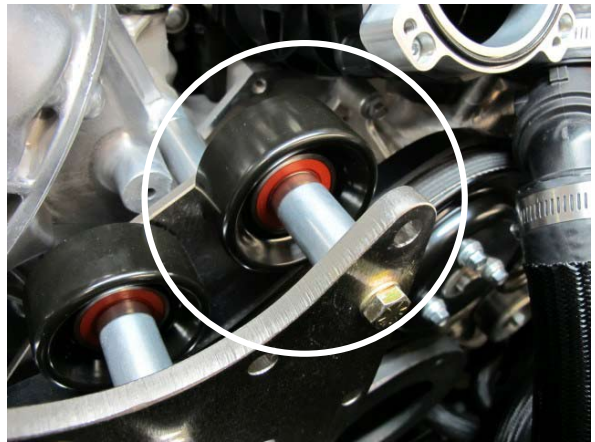
Fig. 2-j: Install previously removed smooth idler pulley
