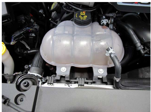
Fig. 1-x: Remove coolant reservoir
