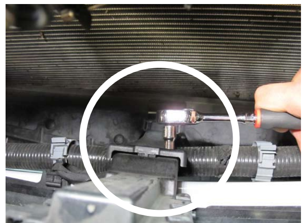
Fig. 1-r: Remove 2x 5.5mm-headed fasteners
