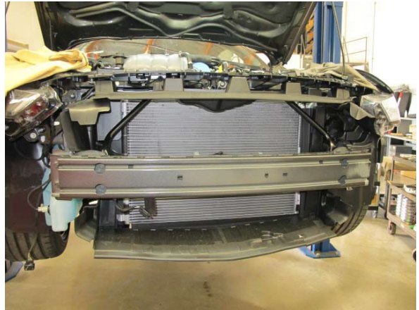
Fig. 1-m: Remove front bumper cover
