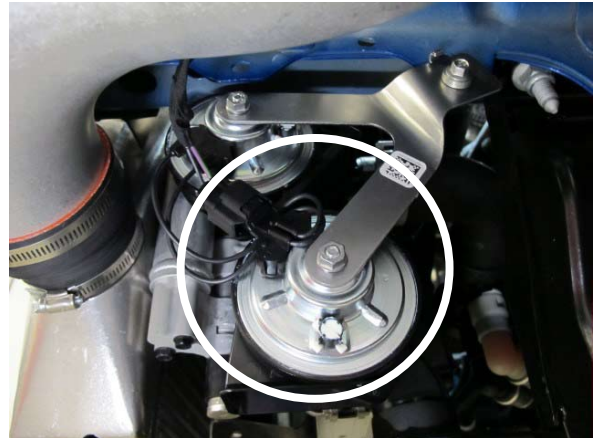
Fig. 6-at: Install horn assembly
