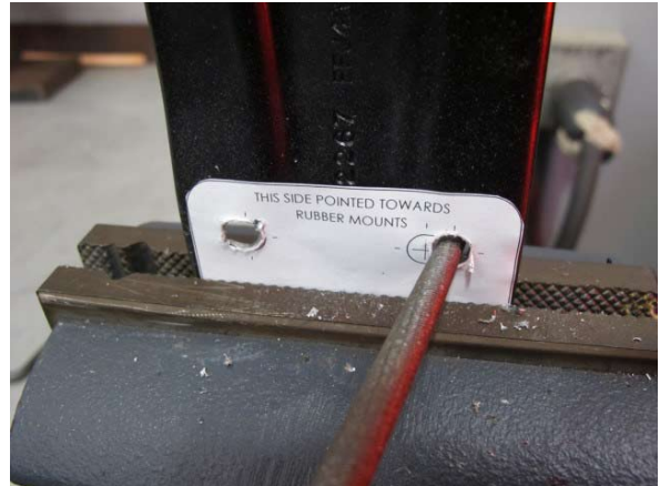
Fig. 4-d: Use round file to slot hole
