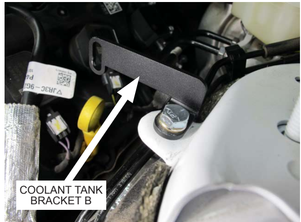
Fig. 4-q: Secure coolant tank bracket B
