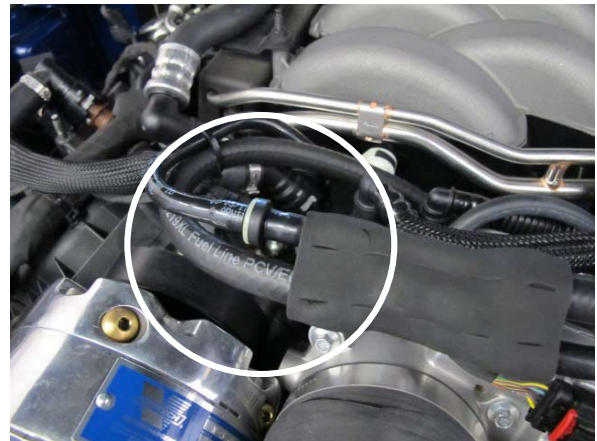
Fig. 7-k: Install 24" length of 3/8" hose
