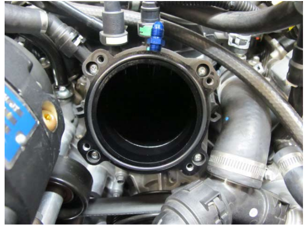
Fig. 6-b: Install throttle body spacer
