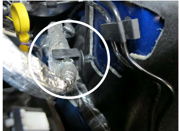
Fig. 4-p: Release EVAP hose from driver side shock tower
