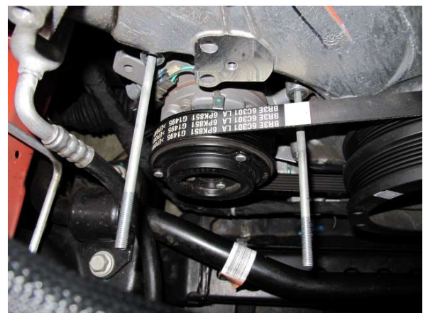
Fig. 2-f: Install threaded studs
