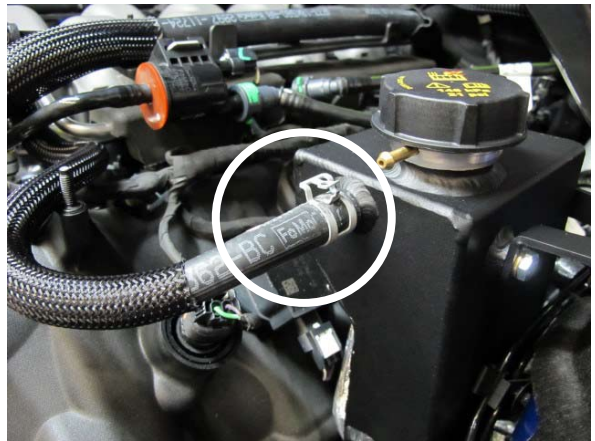
Fig. 4-t: Attach upper OEM molded coolant hose
