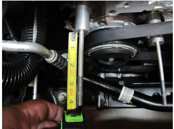
Fig. 2-g: Install 1x 2.058" and 1x 2.146" spacers
