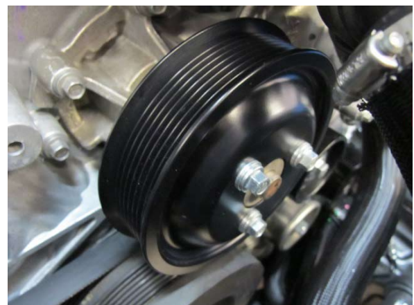
Fig. 2-r: Install 8-rib water pump pulley
