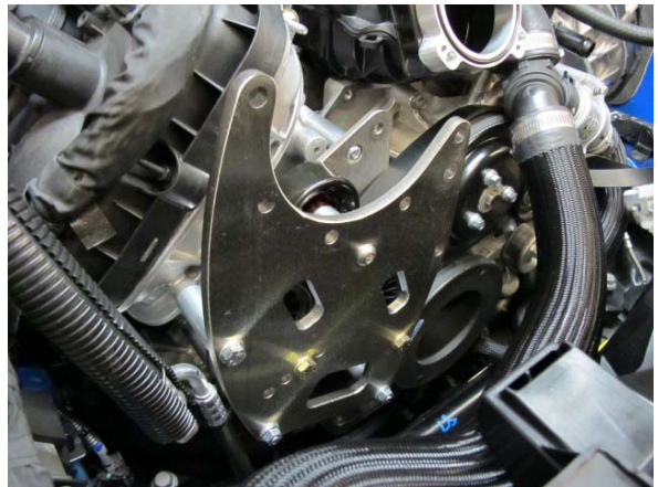
Fig. 2-h: Install 8-Rib drive supercharger mounting bracket assembly
