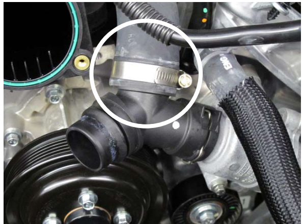
Fig. 4-h: Install #24 hose clamp
