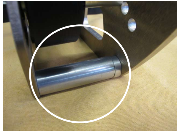
Fig. 2-e: 2x 2.730" spacers and 2x .280" spacers
