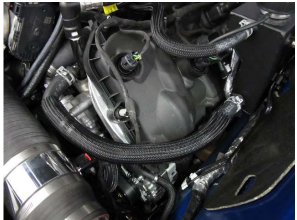
Fig. 4-w: Secure modified OEM 3/4" coolant hose
