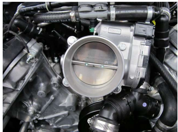
Fig. 6-c: Reinstall throttle body
