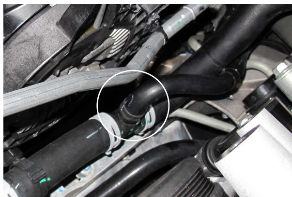
Fig. 5-d: Re-attach Supplemental Radiator Hose
