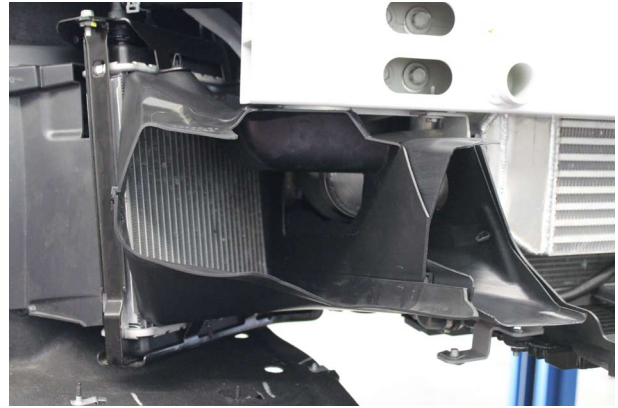
Fig. 8-d: Test Fit Cooling Ducts
