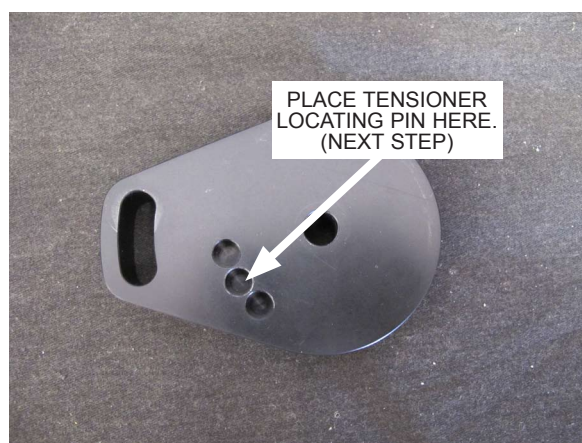
Fig. 6-r: Tensioner Mounting Plate
