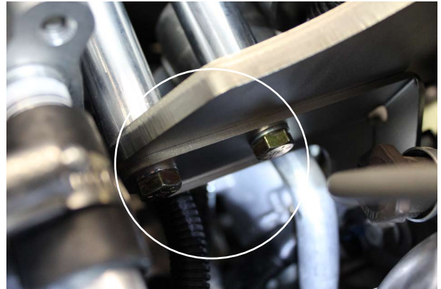
Fig. 6-j: Tighten Rear Support Bracket Screws
