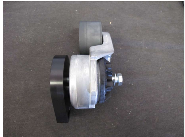
Fig. 6-s: Spring Tensioner & Tensioner Mounting Plate
