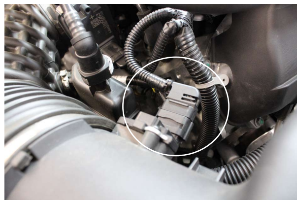
Fig. 1-z: Unplug MAF Sensor
