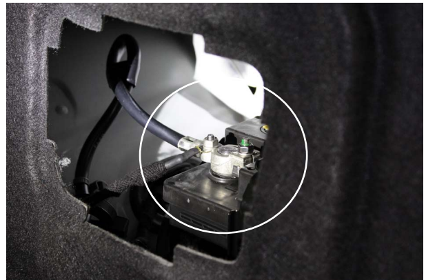
Fig. 1-b: Unplug Negative Battery Terminal
