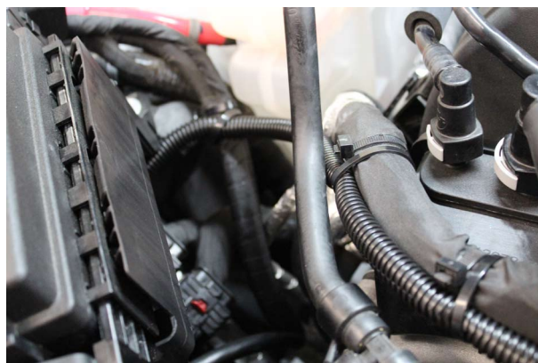
Fig. 8-j: Route MAF Harness Extension Towards Fuse Box
