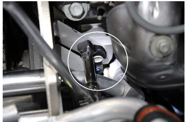
Fig. 6-k: Re-tighten A/C Mount Screw
