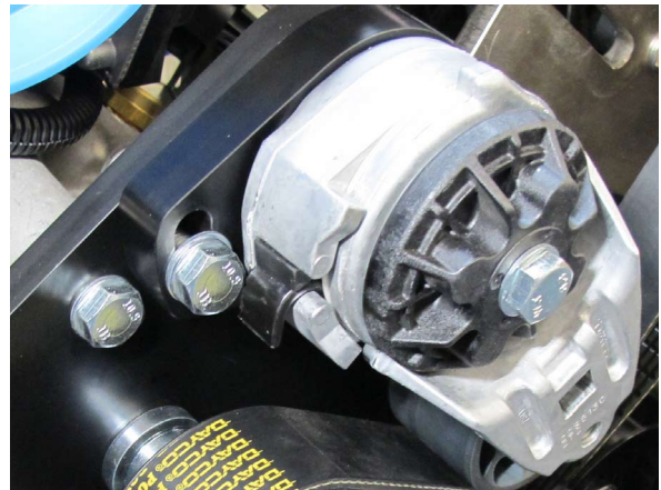
Fig. 6-t: Install Spring Tensioner & Tensioner Mounting Plate
