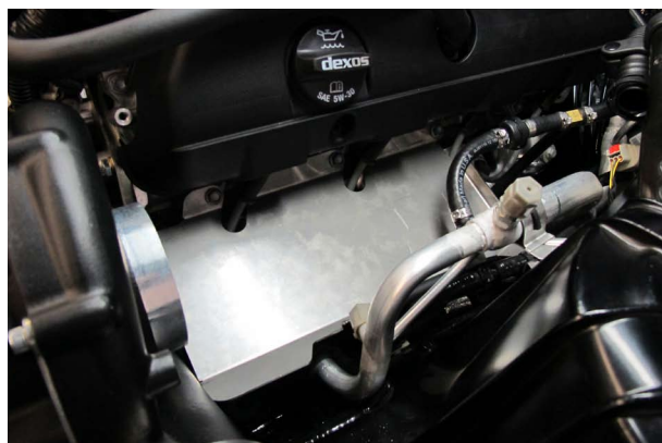
Fig. 10-c: Secure Heat Shield
