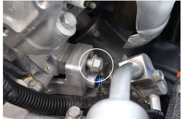
Fig. 6-d: Loosen A/C Mount Screw
