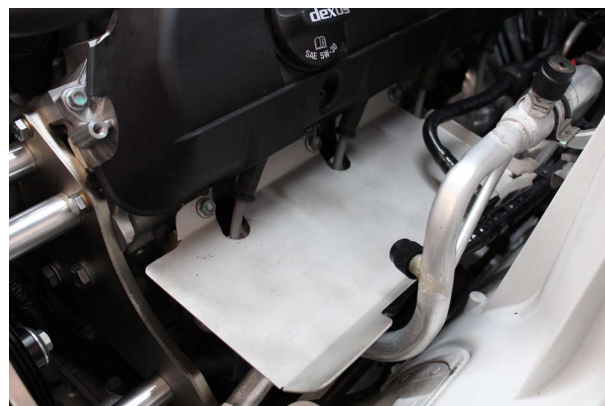
Fig. 10-b: Loosely Attach Heat Shield
