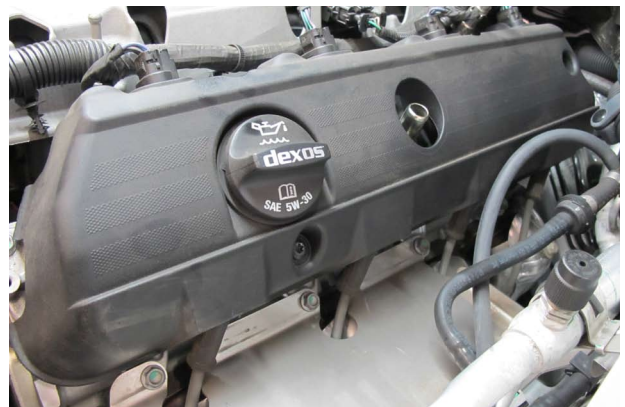
Fig. 6-l: Remove Plastic Engine Cover
