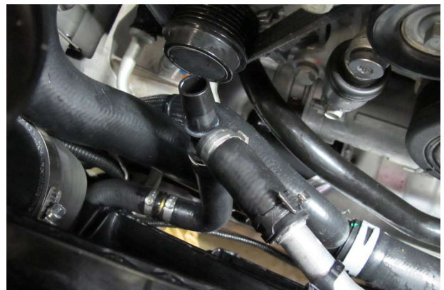
Fig. 5-n: Install Coolant Line Assembly
