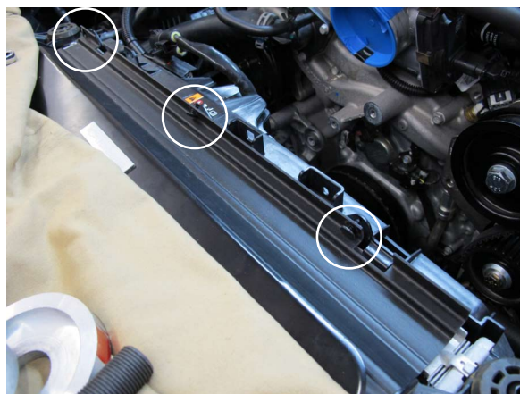
Fig. 3-j: Remove Upper Radiator Shroud
