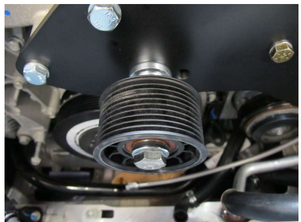
Fig. 6-o: Install 10-Rib Grooved Idler To Idler Plate
