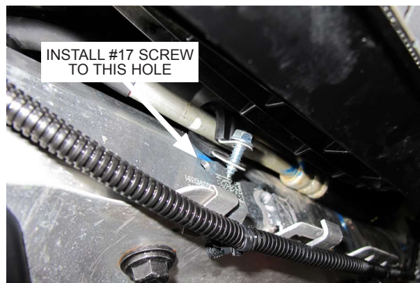
Fig. 5-c: Relocate Transmission Cooler Line
