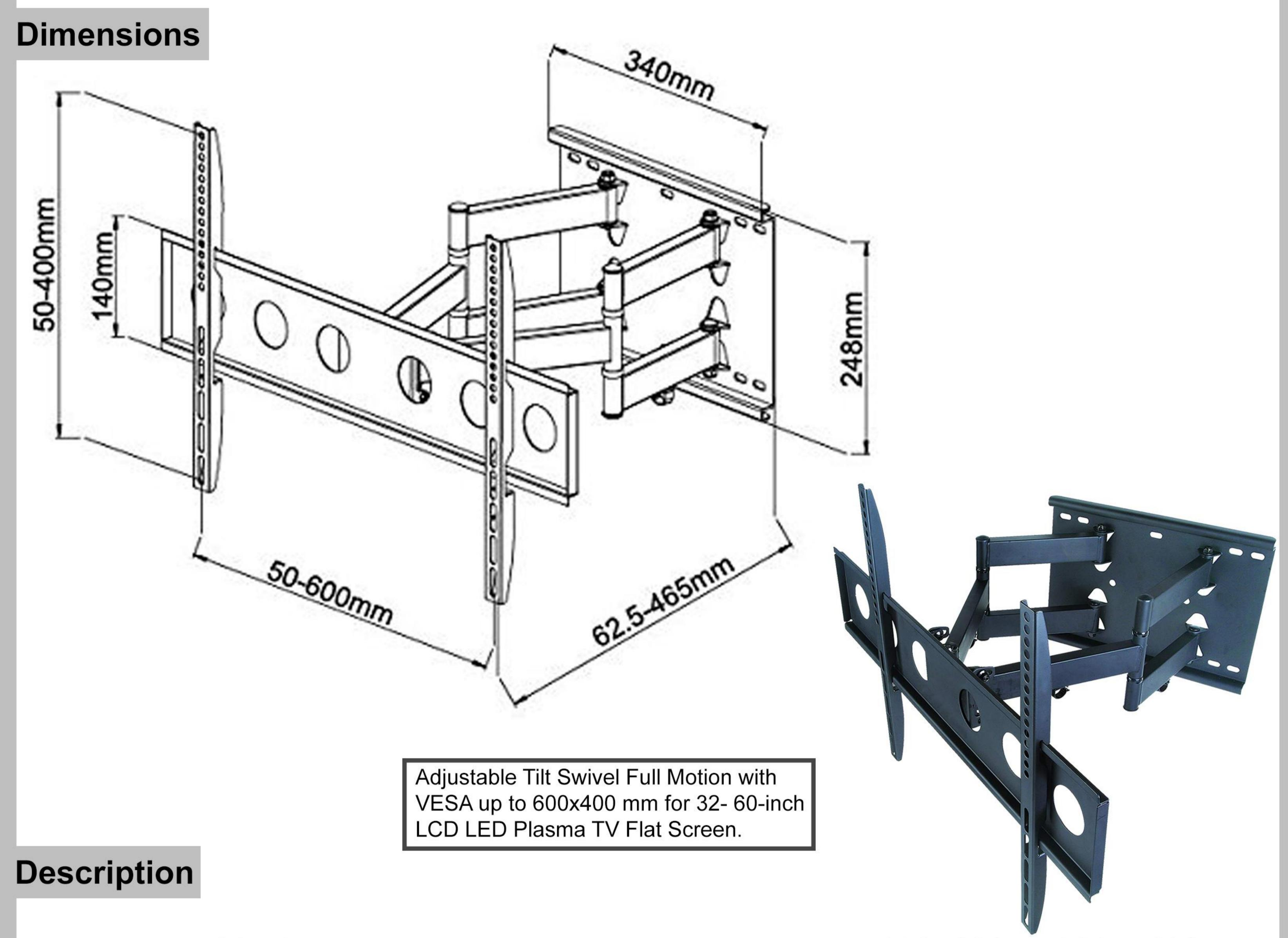
Fits most 32-72 inch TV with mounting hole patterns 200x100 to 600 x 400mm. The wall mount has heavy steel construction, maximum loading capacity to 60 kg. Frontand back telescoping distance (TV to wall distance) is 62.5 cm -46.5 cm.
