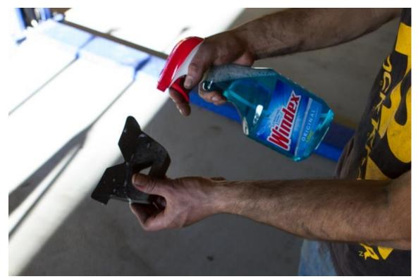
21) Install bump stop into the drop bracket. Install one edge at a time. Bend the bump stop in the middle to get the second side started. Installation can be tricky as the bump stops fit very tightly both in the factory location and in the drop brackets.
