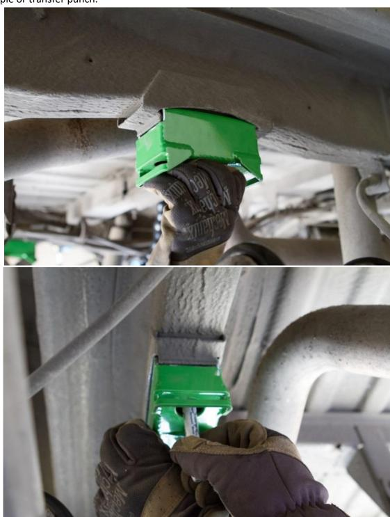
17) Center punch the hole locations and drill with a ¼" (7mm) diameter drill bit.
