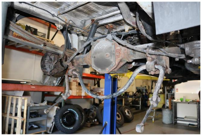
4) On most 3500s, there will be an additional lever connected to the rear axle. Disconnect this lever from the bracket at the axle. Use a 13mm socket / wrench for removal. See image below for reference.
