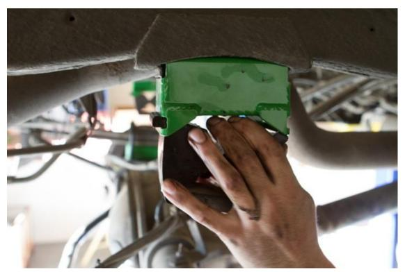
22) Once the second side is started, a screw driver, some wiggling and some additional lubricant will be needed to get the bump stop fully seated in the bracket.
