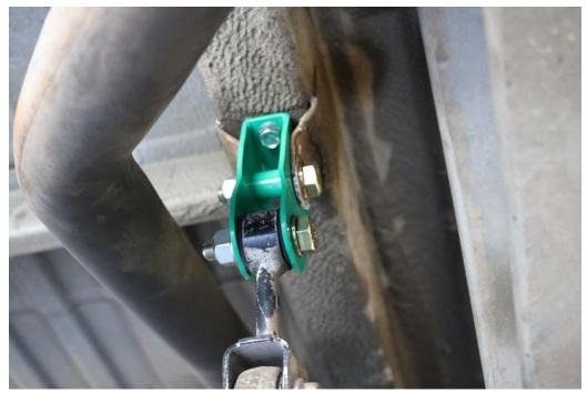
30) Complete rear sway bar installation by securing the sway bar end links to the drop brackets. Use the remaining M12-1.5 x 55mm long bolts provided in the kit with a washer under both the bolt head and stover nut. With a 19mm socket and wrench, torque both upper and lower M12 hardware on the drop bracket to 60 ft-lbs (95 N.m).
