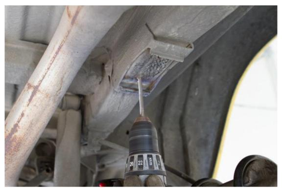
18) With both holes drilled, positions the bump stop drop bracket in place and secure it to the chassis using the  $5/16-18 \times 1''$  long thread cutting screws included with the kit. Use a nut driver or drill with a 1/4'' bit adapter and a 1/4'' socket to install the screw. Try to keep the drill / driver as straight as possible when cutting the threads.
