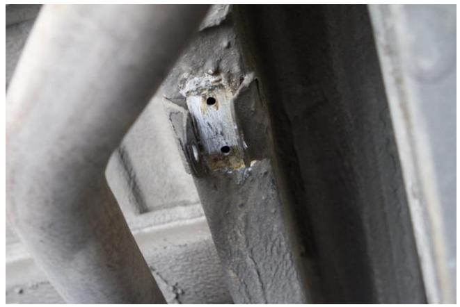
27) Reinstall drop bracket. Again, align with the 12mm bolt provided. Use the  $5/16-18 \times 1''$  long thread cutting screws included with the kit. Use a nut driver or drill with a  $\frac{1}{4}$ " bit adapter and a  $\frac{1}{4}$ " socket to install the screw. Try to keep the drill / driver as straight as possible when cutting the threads.
