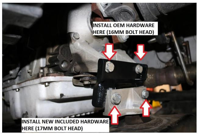
50) Install the factory M10-1.50 bolts in the upper mounting holes to attach the new lift bracket to the transmission. Install the M10-1.50 x 35mm long bolts provided with the kit in the lower mounting hole at the rubber transmission mount. Be sure to use a washer under the bolt head and nylock nut. Snug all hardware but do not fully tighten. Final tightening will occur once the motor mount lift spacers are installed.
