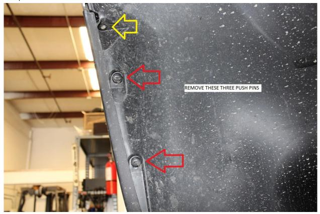
22) Note, the bottom two fasteners (denoted with the red arrows) are the same "cam style" fastener from step 5. The upper fastener (denoted with the yellow arrow) is a standard style push pin which can be removed in two steps. Simply pry up under the push pin head prior to prying underneath the body of the fastener.
