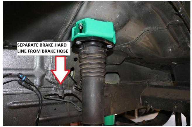
82) Install the front brake line drop bracket as shown below. Use the M12-1.50 x 25mm long bolts provided in the kit. Use a washer under both the nut and the head of the bolt.
