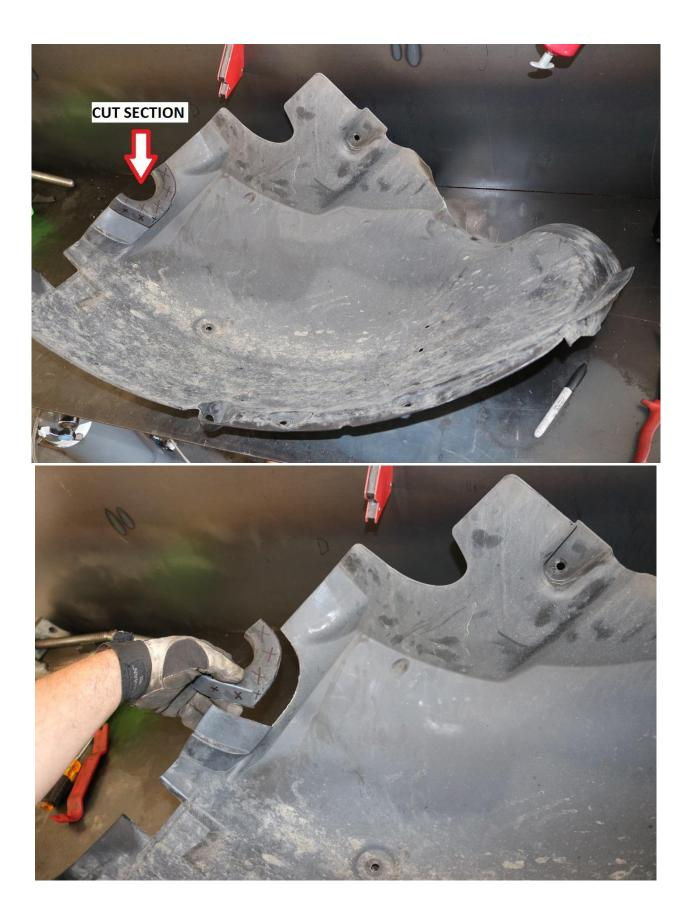
71) The rear half of the fender well liner trimming is very similar. Again, see the images below for reference.
