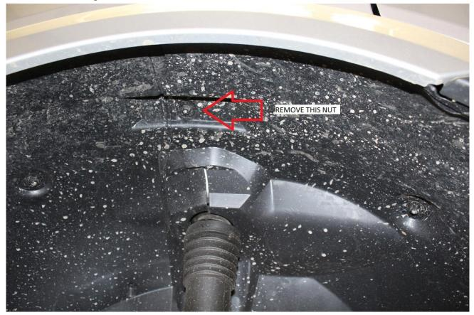
26) Remove the front half of the inner fender well liner by pulling the liner away from the bottom stud as shown.
