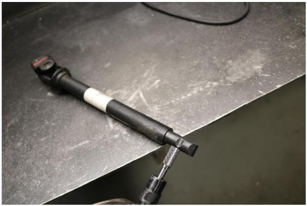
77) Once the pinch bolt can easily be installed, paint any newly exposed areas of metal to prevent corrosion. Assemble the steering shaft extension onto the steering shaft as shown below. Use a small dab of blue Loctite on the threads of the socket cap screw and torque to 18 ft-lbs (24N.m) using a 6mm Allen wrench.
