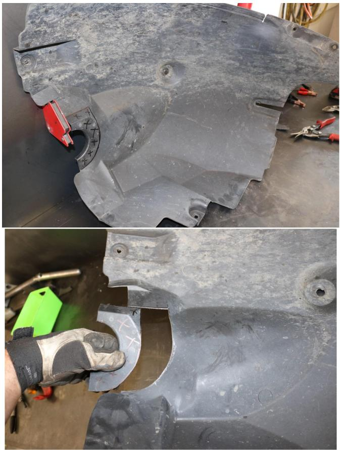
72) Re-install the fender well liners in the reverse order of removal. The trimmed liners should appear as shown below.
