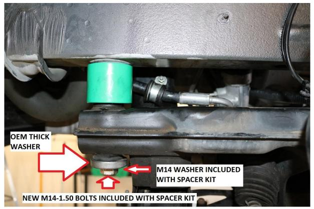
48) Snug all 6 bolts but do not torque at this time. Final torqueing will occur once the motor mount spacers are installed and the engine / transmission support jacks & jack stands can be removed.
