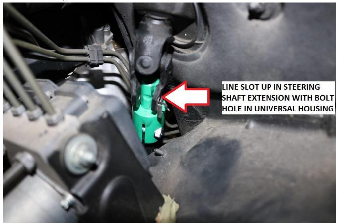
80) Install the bolt, retaining clip and nut removed in step 6 back onto the steering shaft. Use a 13mm socket / wrench and torque to 18 ft-lbs. (24 N.m)
