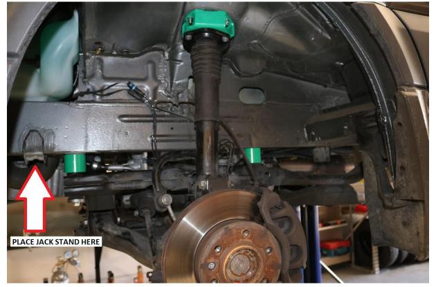
b. If performing this installation on an automobile lift, place lifting point just forward of the gas tank on the vehicle's main chassis section. Mirror this location on the passenger (right hand) side.
