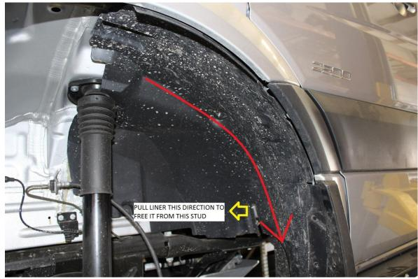
31) The liner should now be able to rotate down and out the direction denoted above with the large red arrow.
