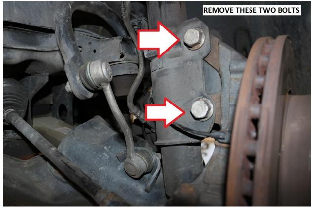
16) With the strut disconnected from the steering knuckle, allow the lower control arm to hang free again. Be careful to slowly lower the knuckle out of the strut. Be sure the wheel speed sensor wire is not strained.
