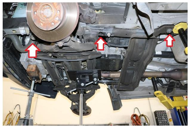
44) Prepare the spacers and new sub frame attachment bolts. The image below shows where each bolt / spacer is designed to be installed. It is critical to use the correct bolts / spacers in their corresponding locations.
