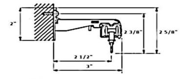
Place the front lip of the track into the bracket as shown, applying upward pressure until the track clicks into the bracket. A bracket should be used near the splice for support.
