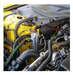
The clean line will route from the front of the catch can to the throttle body using one of the OEM connectors you removed in the previous step. The dirty line routes from the top of the catch can to the oil pan using the other OEM connector.
