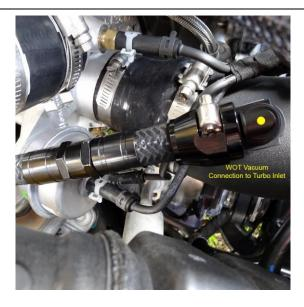
Connect the WOT vacuum line from the back of the can to the quick connect fitting you just installed on the turbo inlet.
