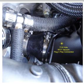
Drill a 7/16" hole in the turbo inlet tube and screw in the billet quick connect fitting. Make sure to keep any plastic from getting into the tube by either removing the tube for drilling or using grease on the drill bit.
