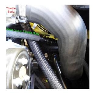
Proper hose routing of the clean line to throttle body. With everything in place tighten all clamps on billet ends.
