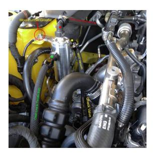
Mount the catch can to the passenger side strut tower under the ground strap bolt as shown. Remove the OEM line from the throttle body to the oil pan. Heat the ends of the line to remove the OEM connectors.
