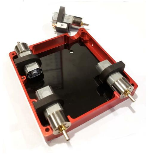
Align the motors with the outside edge of the chassis:
