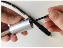
**4.** Inside the flexible driver's hood, you'll find the inner drive shaft - pull enough of it out to be able to work comfortably.
