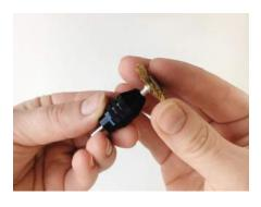
**1.** Insert your chosen accessory in the adjustable chuck. You can see a picture of the adjustable chuck on page 11.
