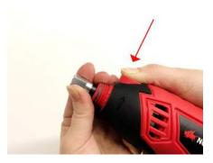
**3.** Push down the shaft lock button (see page 9) to fully tighten the cap nut in place.
