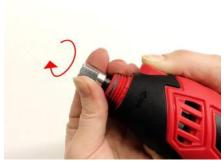
2. Take the hex cap nut and screw it onto the rotating part of the tool. You can see a photo of the hex cap nut on page 11.
