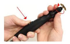
**3.** Insert the adjustable chuck with the chosen accessory onto the flexible driver, and rotate clockwise to securely fasten, while keeping the shaft lock button pressed. When tight, release the shaft lock button and start work!
