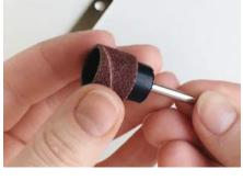
1. Loosen (not remove) the small screw on top of the black rubber sanding drum with the screwdriver on the back of the wrench. This will contract the rubber, so you can slide the sanding band onto the drum. Picture of the wrench/screwdriver can be found on page 19, sanding bands and drums on page 18.
