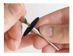
**5.** Use the screwdriver end of the wrench to tighten the mandrel to secure the disk firmly in place, so it does not wobble. Do not to over tighten as the disc can crack.
