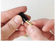
**2.** Put the accessory aside for now, and insert the properly sized collet inside the collet nut. To see the difference between the collet nut and the chuck nut, flip back to page 11.
