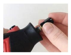
**3.** Put the collet nut with the collet on the rotary tool shaft.
