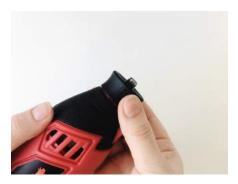
**1.** First, unplug the tool from the power supply and remove any attachments and housing caps from the rotating tip of the tool.
