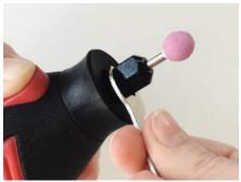
**6.** To make sure that the collet nut is as tight as it can be (you don't want to suddenly have your cutting discs flying off), take the wrench that came in the rotary tool kit, and tighten the nut. And yes, keep the shaft lock button pressed down while doing so - it prevents the shaft from rotating while you're adjusting the nut. If you want to see what the wrench looks like to locate it in your kit, flip back to page 19.
