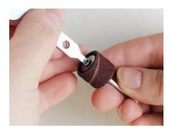
**3.** Tighten the screw on top of the sanding drum with the screwdriver. This will expand the rubber, so the sanding band won't slide off the drum.
