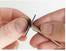
**4.** Rotate the small screw with the disc attached back on the mandrel shank.
