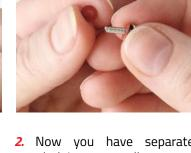
1. Loosen the small screw on top of the cut-off & sanding disc mandrel with the included screwdriver. You can see the cut-off & sanding disc mandrel on pages 15 or 18. A picture of the wrench/screwdriver is on page 19.
