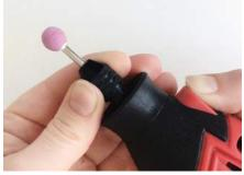
1. Choose your accessory, and insert it into the adjustable chuck nut. To see the difference between the chuck nut and the collet nut, flip back to page 11.
