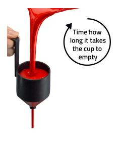
Place your finger over the hole of the included flow cup and fill it to the brim with your chosen material. At the same time, release your finger from the hole, and start the timer. Stop the clock when the flow cup has completely drained of paint.
