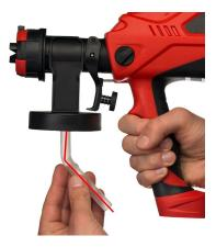
If painting objects that are on or close to floor level, it's best to position the suction tube *away* from the body of the paint sprayer.
