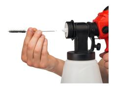
2. Use a pointy object (a screwdriver or the back of the included cleaning brush works great!) to remove the sprayer nozzle tip.
