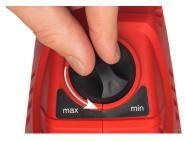
For thicker paints (more than 50 DIN/s) - turn the dial clockwise to maximum for when you need to quickly cover a large area. For thinner paints (less than 50 DIN/s) - turn the dial anti-clockwise to minimum for when you need a more steady, deliberate spray.
