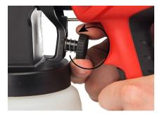
For thinner paints (less than 50 DIN/s) - turn the dial anti-clockwise (loose against the trigger) to decrease the amount of paint dispersed by the sprayer.
