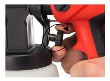
For thicker paints (more than 50 DIN/s) - turn the dial clockwise (tight against the trigger) to increase the amount of paint dispersed by the sprayer.
