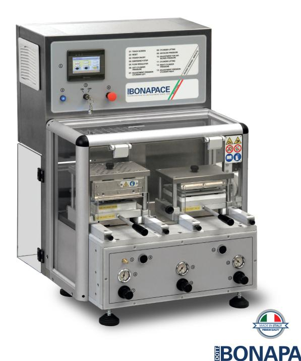
IN-PACK IS THE PNEUMATIC BLISTERING MACHINE, IDEAL FOR CLINICAL TRIALS, STABILITY TESTING, PACK DEVELOPMENT AND LOW VOLUME PRODUCTION FOR LABORATORY OR CHEMIST'S SHOP. THE MACHINE IS THERMOFORMING, SEALING, CODING AND CUTTING BLISTERS IN PVC/ALU AND ALU/ALU.
