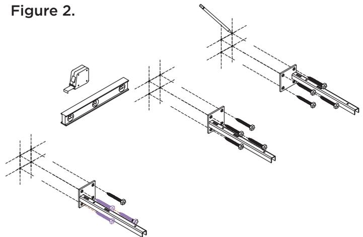
**Step 3:** Secure each wall bracket to the wall with the bolts provided.
