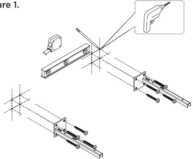
**Step 2:** Place the left wall bracket on the left outline and mark the location of the bolt openings.
