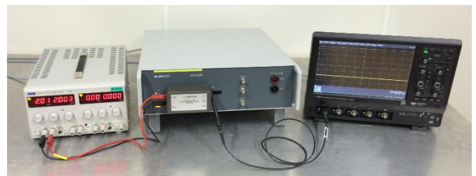
Figure 8.14: Example calibration setup with PFM 200N100.1, CA LV124-D1R and Scope. Set the external voltage source to 2.00V with 2.0A current limit setting.
