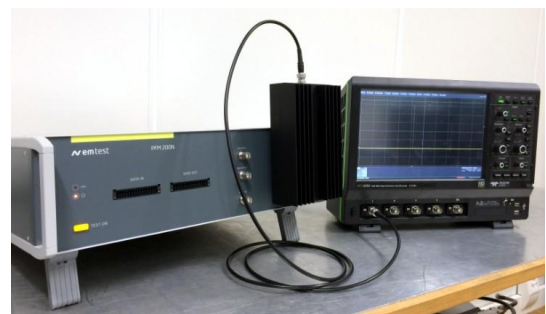
Figure 7.15: Example Verification setup with PFM 200N100.1, CA LV124-P1R and Scope
