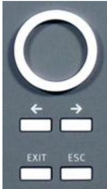
The selected parameter is blinking and can be changed by turning the knob (incr./decr.).
