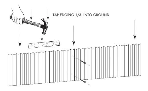
**INSTALLATION OPTION 2:** Reinforce with Wooden Stakes
