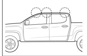
**Side View:** Hook the Stud Housing on the Track as shown. Care is needed as to not damage the body work of the vehicle.
