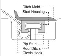
**Side View:** Carefully flex the Stud Housing over the Pip Stud. Complete this step for each Pip to release the Ditch Mold.
