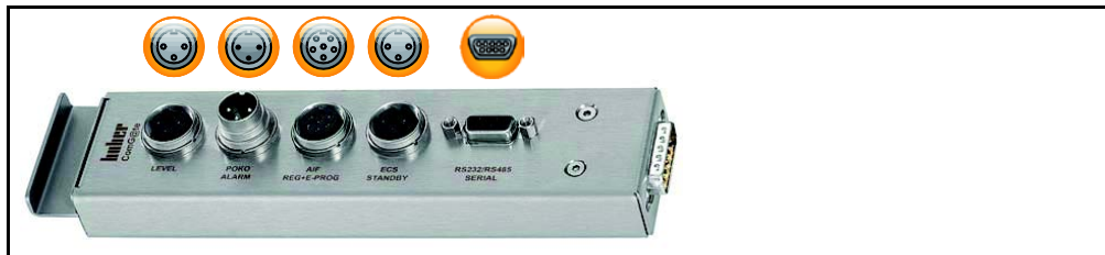
Com.G@te external interfaces: LEVEL, POKO, AIF, ECS, RS232/RS485 (left to right).
