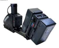
Generally we use the battery in pairs, generating (nominally) 29.6VDC. It's best to use batteries that are roughly equally charged. Both batteries power the 14.4 volt DC to DC converter nestled between the batteries.
