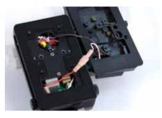
Normally, the red stripe wire is connected to the other red stripe wire (for 24 volts and 14 volts via the converter or 12 volts via the rear battery). Carefully pull apart the connectors, and pull out the solid red wire. Connect the solid red wire to the red stripe wire. This will connect the two batteries in parallel and disconnect the converter from the circuit. 24 volts is not possible with only two batteries in this mode.
