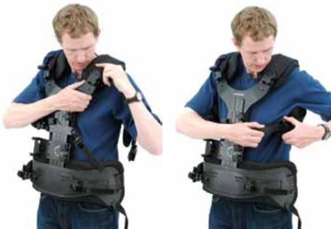
The chest pads are snugged up next. You should be able to breathe a little, but the vest should not be able to slip forward and down. Diaphragmatic breathing (like a baby) works best.
