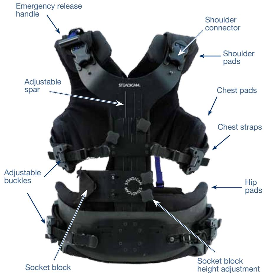
Note: The vest must be properly adjusted for the emergency release system to work. The emergency release line (blue) should be taught and both cross back straps disconnected. See p312-313 of *The Steadicam<sup>®</sup> Operator's Handbook*, for the quick release demo.
