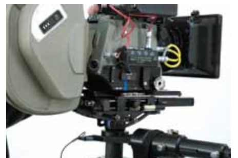
Dovetail locking lever fully open.
