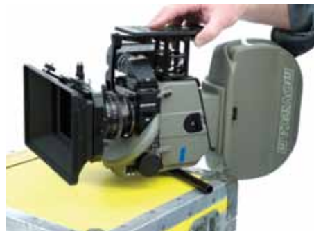
Finding the camera's fore-aft center of gravity.
