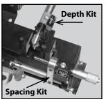
Upgrade turns your Model 200 Key Machine into a code cutter worth hundreds of dollars, allowing you to control both the depth and the spacing on your Model 200 machine with the accuracy of a direct read digital micrometer. These two direct read digital micrometers are only found on key machines that cost hundreds, if not thousands, of dollars more. These are non-electronic digital micrometers.
