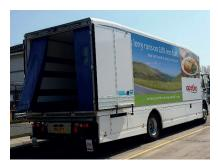
"The truck fitted with the Back-Stop system recorded a 58% improvement in terms of temperature retention when compared with the vehicle fitted with the original plastic curtain system." – apetito
